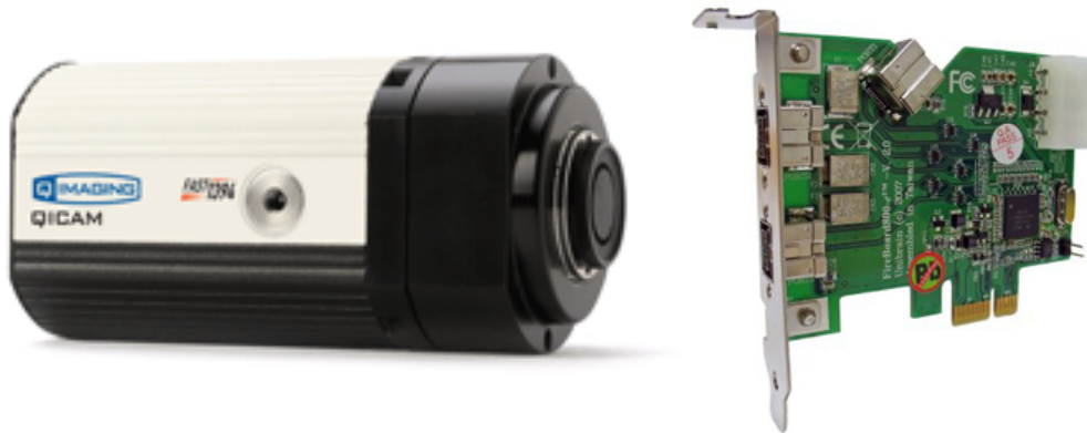
Figure 192. The QImaging QICAM which provides a cost effective entry level digital CCD camera.
