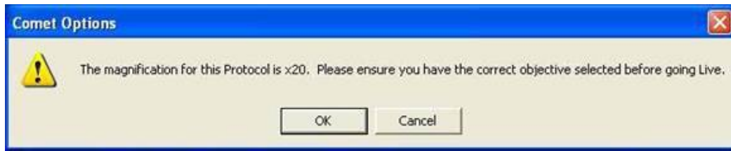
Figure 157. A Magnification reminder is shown – Make sure you have the correct objective in place and make sure the microscope beam-splitter is in the correct position to send an image to the camera.
