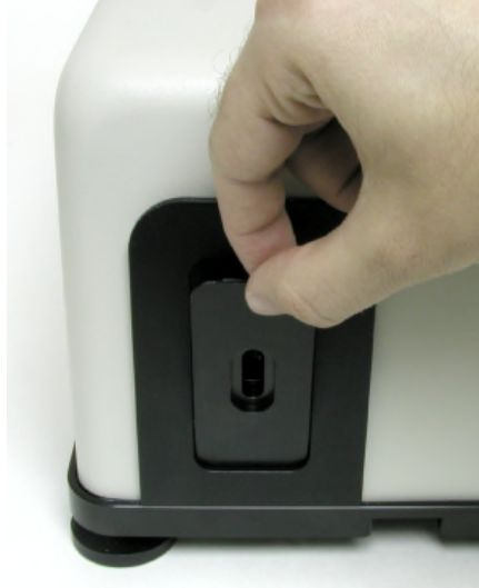
Figure 4-7. Installing the input adapter.
