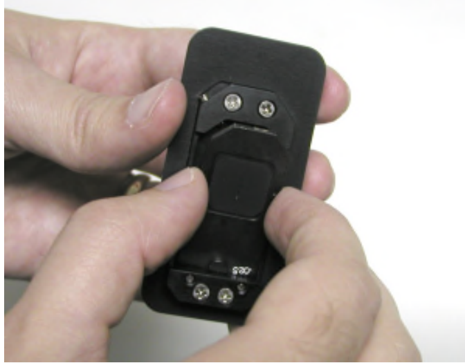
Figure 4-13. Inserting a slit into an input adapter.
