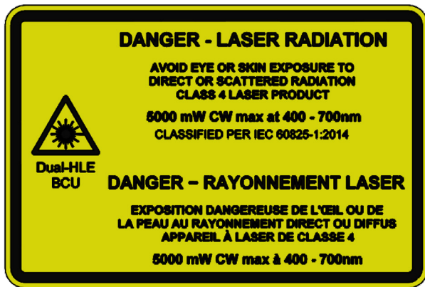
Figure 2: Dual-HLE BCU Class 4 Labels, location on the top of the BCU. These labels are not provided for a BCU driven by a single HLE as the label on the HLE is sufficient to cover it. However, in a dual-HLE configuration the output of the BCU is a combination of HLE outputs and so the combined power must be given.
