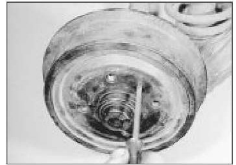
9.3a Removing a brake drum securing screw
