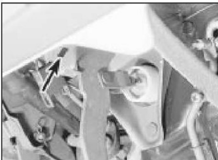
17.1 Stop-lamp switch 'keyhole' mounting (arrowed)
