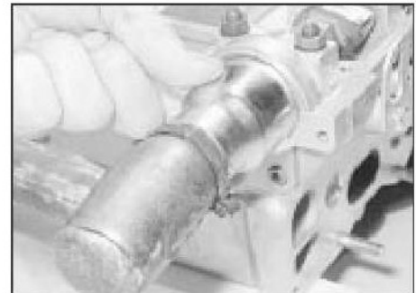
9.4b Seating a camshaft oil seal
