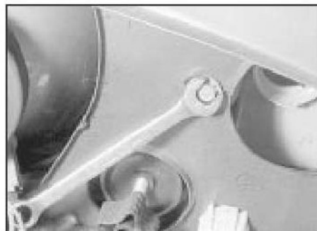
12.2a Undoing a direction indicator lens screw
