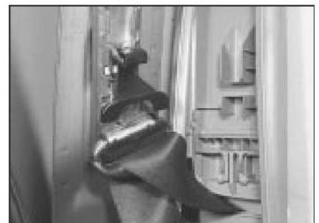
37.6a Front seat belt adjustable top mounting
