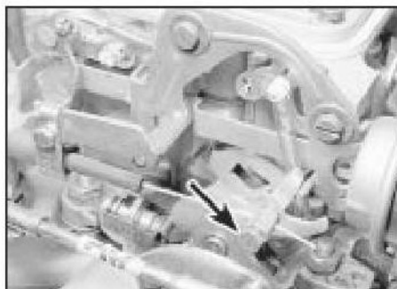
10.5 Choke cable inner clamp screw (arrowed)
