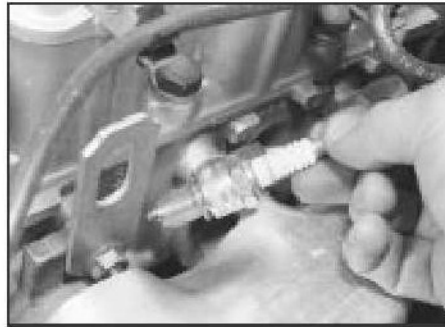
7.5 Removing a spark plug - 1.6 litre engine shown
