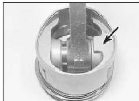
15.1 Large land (arrowed) faces the flywheel end of the engine
