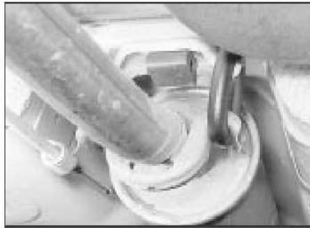
27.4b Exhaust system rubber mounting ring
