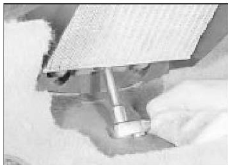
9.17a Removing the heater matrix lower screw
