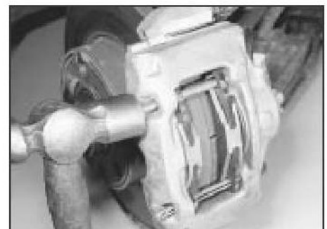
4.10a Inserting disc pad pin
