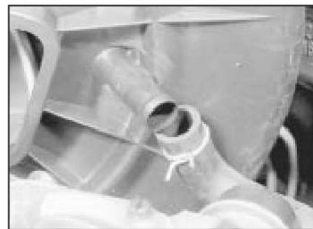
3.2c Air cleaner hose connection
