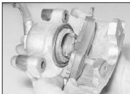
4.21a ... then unclip the inboard pad from the caliper piston ...
