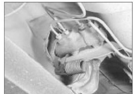
14.8 Load-dependent pressure regulating valve, spring and bracket - Estate and Van models
