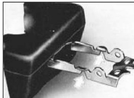
23.23 Float adjustment points (arrowed)
