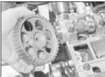
10.3b Removing a camshaft sprocket
