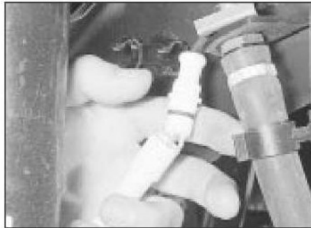
22.3b Separating a front sensor connector
