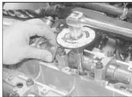
11.24b Angle tightening a cylinder head bolt
