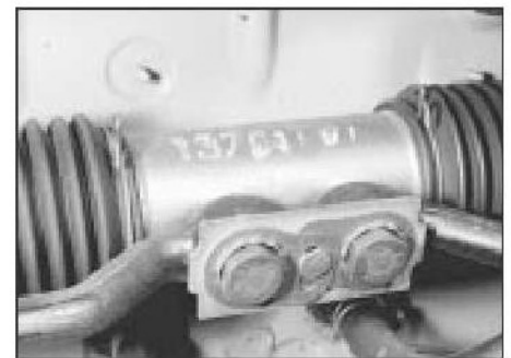
27.4 Tie-rod connection to steering rack
