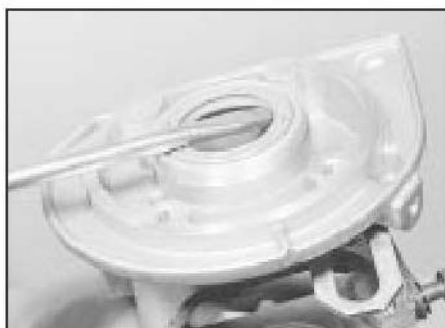
9.8a Prising out the camshaft housing oil seal
