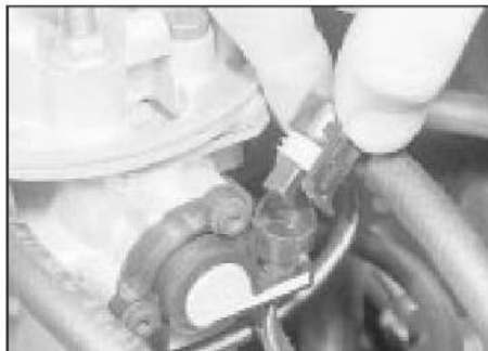
11.3a Detach the wiring connector from the throttle valve potentiometer
