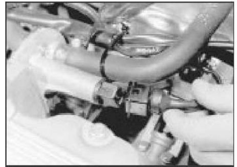
13.3d Unplugging the auxiliary air valve
