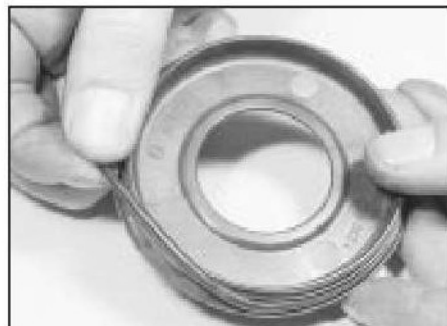
3.27 Renewing the insulator sealing ring
