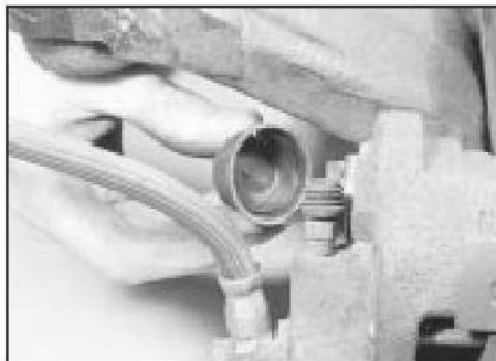
10.6a On the GMF caliper, remove the caliper bolt caps . . .
