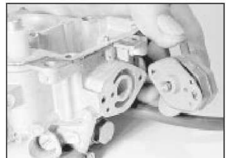
21.6 Removing the part-load enrichment device
