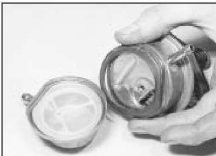
12.2 Removing the fuel pump cover, filter and rubber seal - carburettor models
