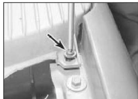
11.3a Wind deflector screw at the wing
