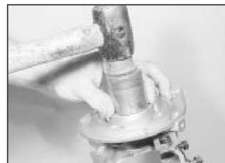
9.8b Fitting a new camshaft housing oil seal
