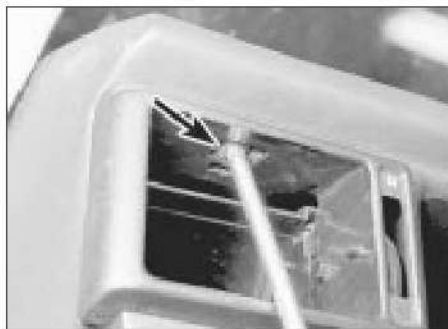
10.2 Removing a swivelling vent housing securing screw
