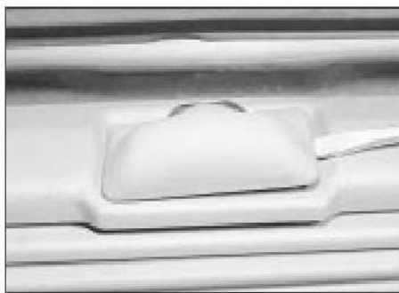
11.22 Prising out the number plate lamp
