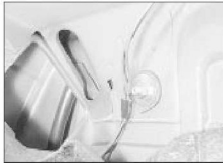
33.3e Rear seat backrest catch retaining nut - Saloon
