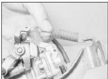
19.3 Removing the throttle return spring
