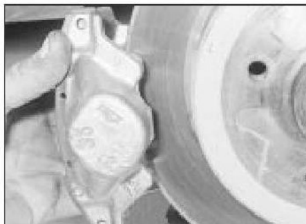
11.5 Removing the rear caliper
