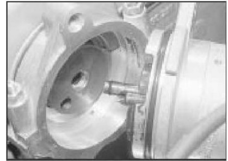
3.17 . . . and remove the distributor
