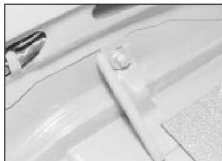
9.2 Rear trim panel securing nut
