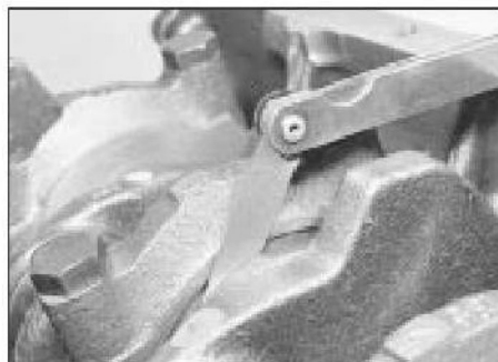
20.19 Checking crankshaft endfloat
