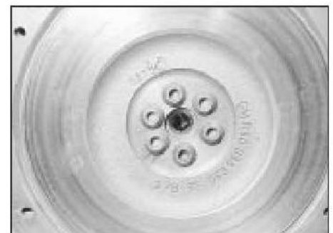
16.4 Flywheel retaining bolts are socket-headed
