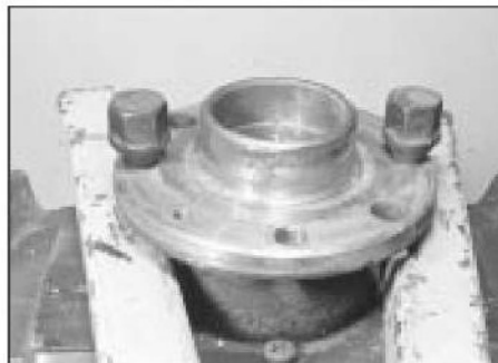
3.3a Removing the hub from the carrier
