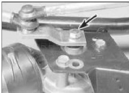
20.8a Wiper motor spindle nut (arrowed)
