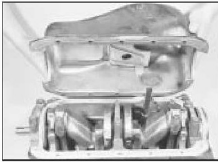
11.9 Refitting the sump
