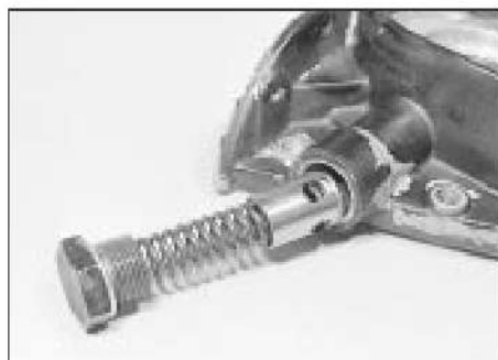
14.5 Oil pressure regulator valve components
