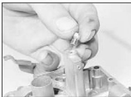
21.10 Removing the main jet
