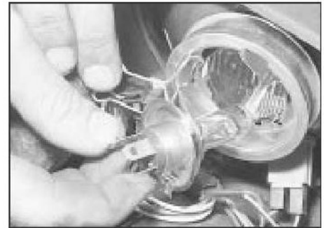
11.3 Removing a headlamp bulb
