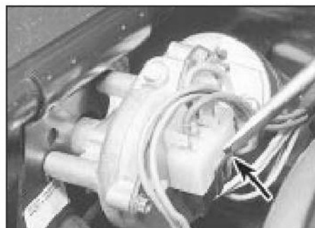
20.6 Releasing the wiper motor electrical plug
