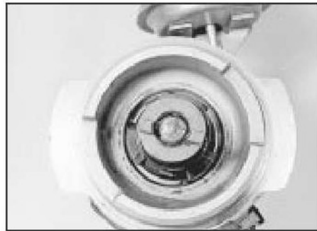
3.19b . . . causing the drive coupling to be aligned like this . . .
