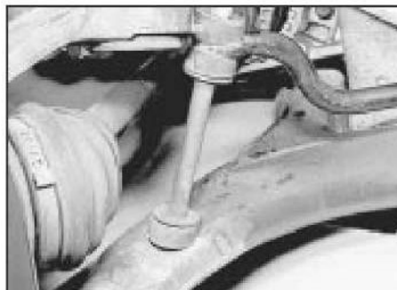
8.2 Front anti-roll bar end link
