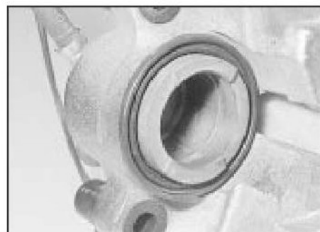
4.23 Prior to fitting the pads, ensure that the caliper steps are positioned as shown
