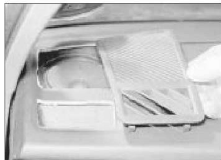
10.1 Removing an end grille and speaker
