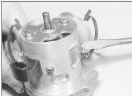
4.16a Removing a vacuum unit retaining screw
