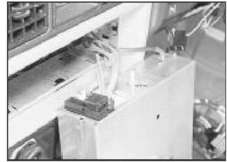
25.2b Removing the radio from its aperture
