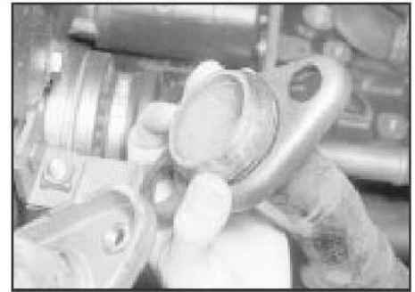
27.5 Graphite sealing ring fitted at the flexible joint
