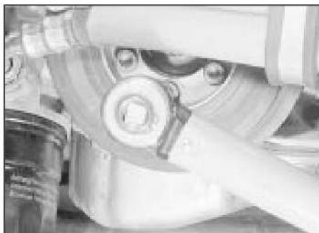
7.14 Tightening one of the crankshaft pulley screws
