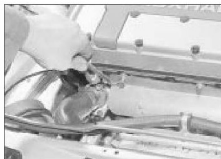
14.3 Removing an exhaust manifold heat shield bolt
