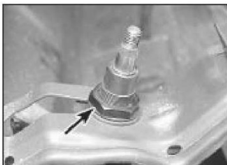
20.4 Wiper spindle clamp nut (arrowed)
