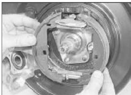
20.4 Removing the handbrake shoe assembly
