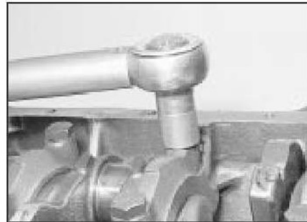
20.16b Tightening a main bearing cap bolt
