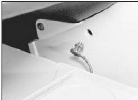
36.1 Glovebox check strap disconnected
