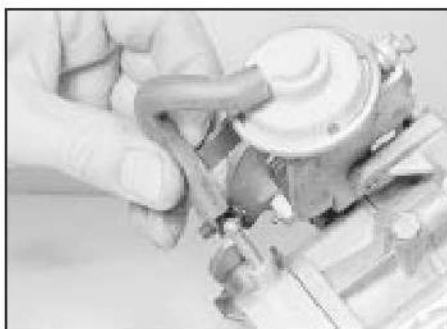
19.4 Disconnecting the vacuum hose
