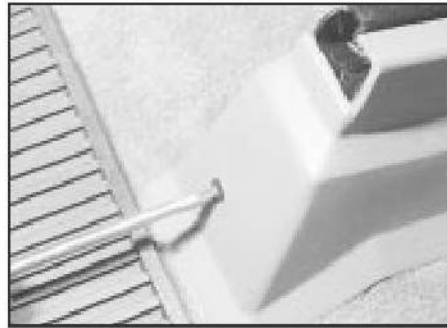
31.1 Seat rail trim removal
