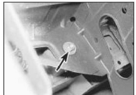
8.3 Front trim panel securing nut (arrowed)
