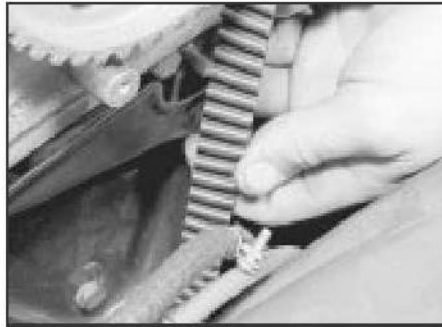
7.24 Checking the belt tension by twisting it between the water pump and camshaft sprockets
