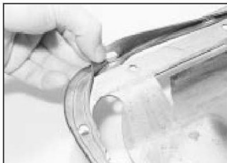
12.7b . . . while this one has one double-sided rubber gasket
