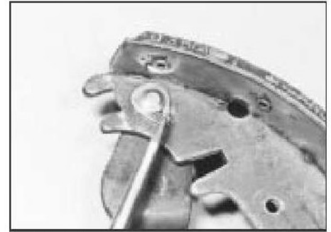
6.16 Handbrake lever secured by pin
