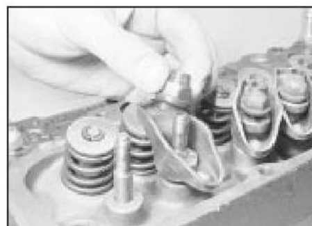
9.25 Fit the nut with the self-locking collar uppermost
