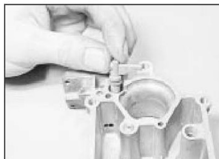
19.11 Removing the fuel discharge nozzle
