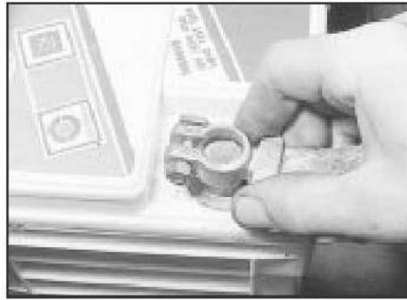
4.2 Disconnect the battery negative terminal first
