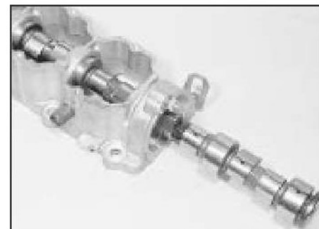
9.6 Removing the camshaft from the housing
