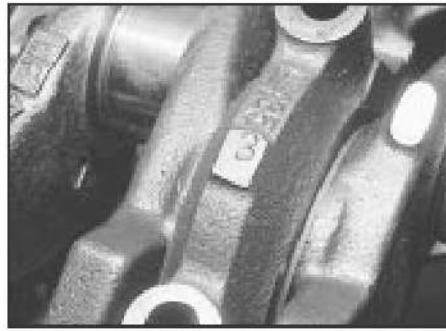
20.3 Identification number on No 3 main bearing cap
