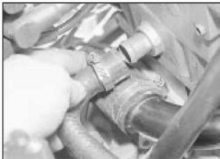
11.11 Disconnecting the heater hose from the cylinder head
