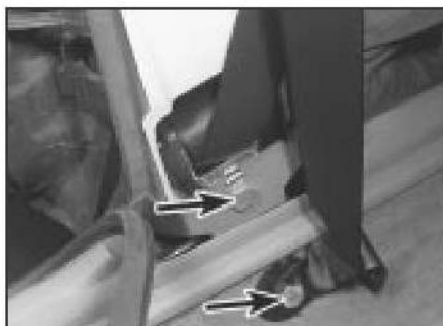
37.5 Front seat belt inertia reel and lower mounting bolts (arrowed)
