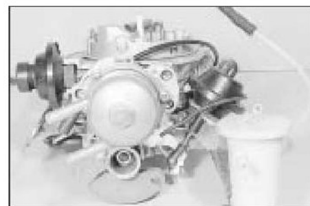
22.2b 2E3 carburettor - choke cover side view
