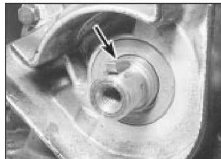
13.2b Woodruff key (arrowed) in crankshaft nose
