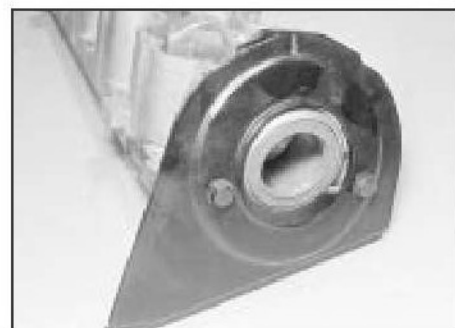
9.7 Camshaft belt cover backplate (1.3 litre engine shown)
