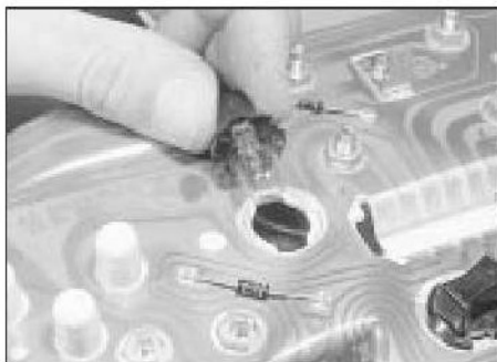
11.27 Removing an instrument panel bulb
