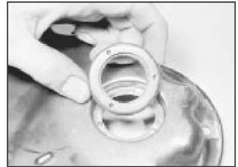
14.14b ... and refit the holder and seal to the timing cover
