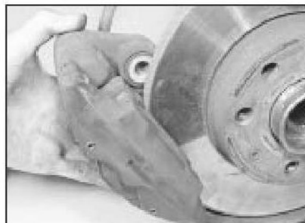
10.6c . . . and remove the caliper
