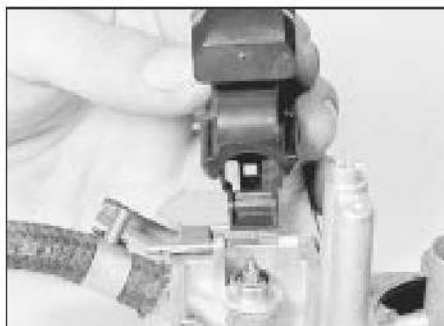
21.9a Removing the float ...
