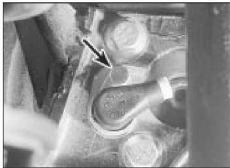
22.2a ABS rear wheel speed sensor on brake backplate securing screw arrowed
