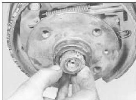
10.6a Fit the outer bearing race . . .
