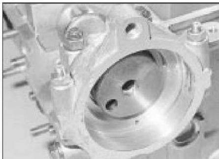
10.7 Distributor housing bearing cap has two extra nuts
