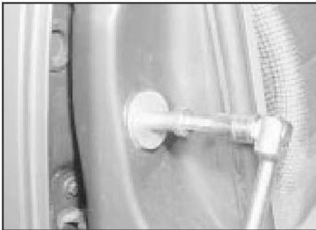
13.4 Adjusting a door lock striker
