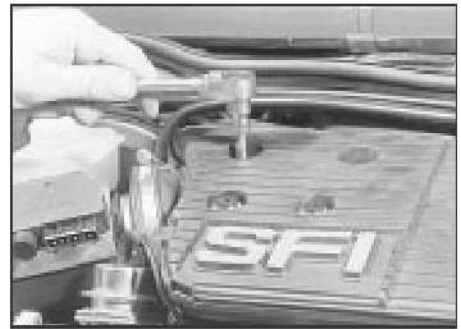
12.77 Removing a pre-volume chamber screw
