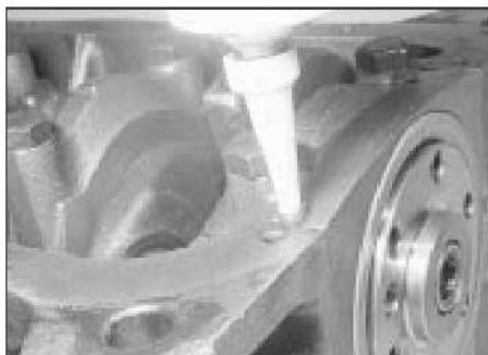
20.17 Inject jointing compound into the cap side grooves
