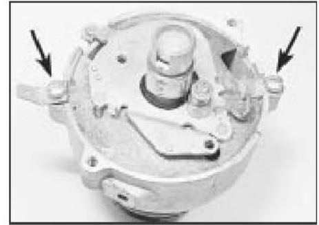
7.7 Undo the baseplate retaining screws (arrowed)
