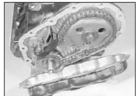
14.21 Refitting the timing cover
