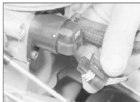
11.11a Detach the wiring connector . . .
