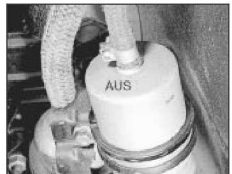
25.4 Fuel filter directional marking
