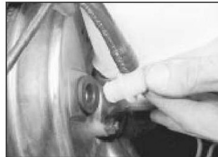
15.3 Brake servo vacuum connection at servo
