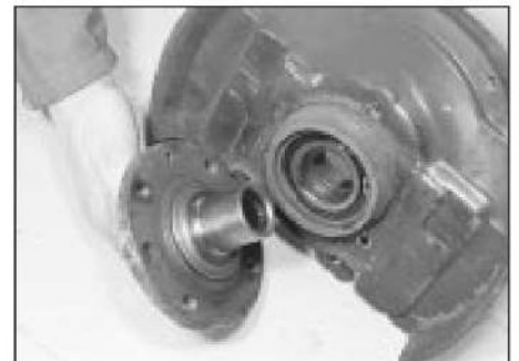
3.3b Hub removed from the carrier
