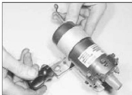
6.4b Undoing the coil clamp screw and nut
