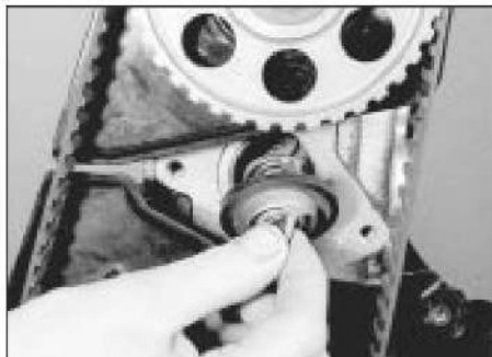
4.7 . . . and withdraw the thermostat from its recess - 1.3 litre model
