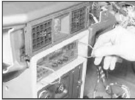
25.2a Inserting the special clips for radio removal
