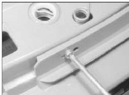
8.2 Undoing a front trim panel screw
