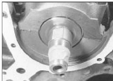
13.6 Tape the crankshaft nose
