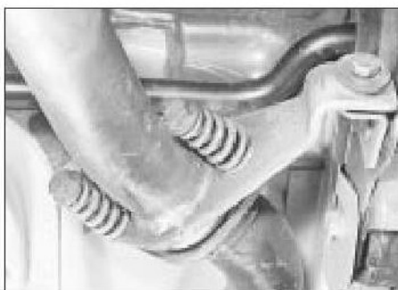
14.5 Manifold-to-exhaust system joint and bracket
