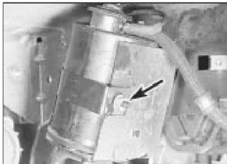
12.98a Canister clamp nut (arrowed)
