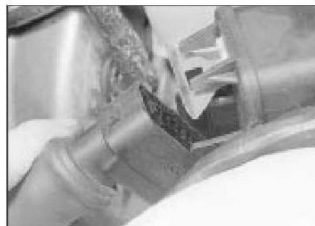
7.7 Disconnecting the control unit wiring plug - later 1.8 litre model
