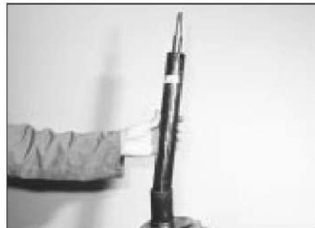
4.7 Removing the shock absorber cartridge
