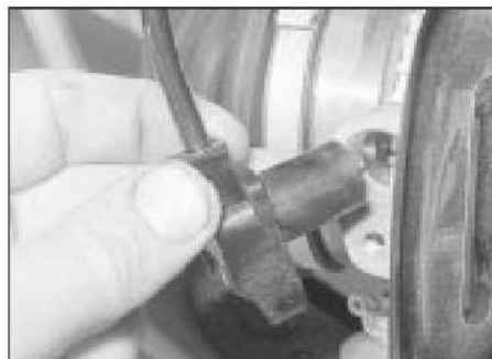
22.2c Removing a front wheel speed sensor
