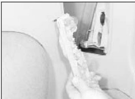
11.16b Rear lamp cluster bulbs and holder
