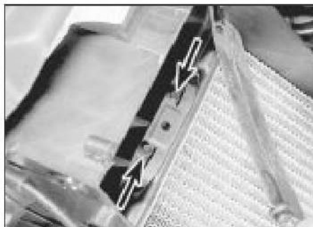
9.17b Heater matrix upper securing screws (arrowed)
