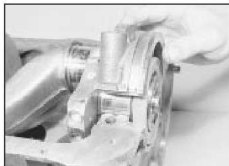
20.16 Fitting the rear main bearing cap
