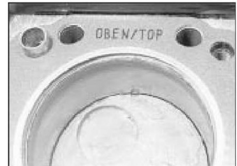
8.22 Head gasket must be fitted with the word OBEH (or TOP) uppermost
