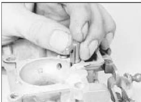
21.8 Removing the accelerator pump delivery tube
