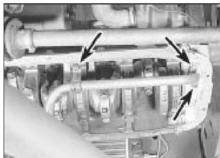
13.4 Oil pick-up pipe retaining bolts (arrowed)
