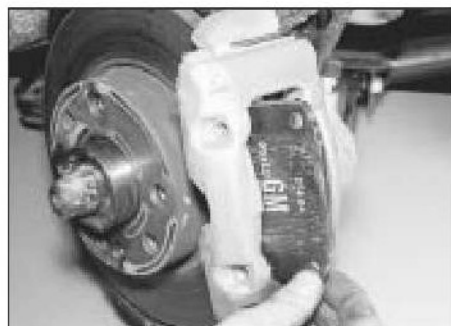
4.5 Removing the outboard pad
