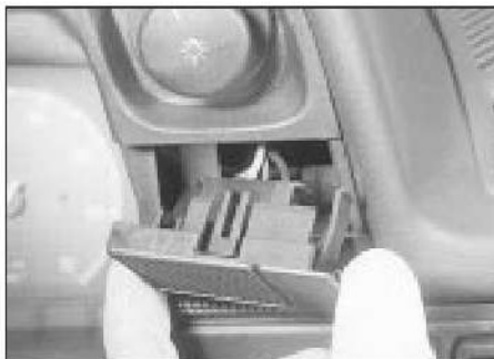
4.5 Removing a foglamp switch
