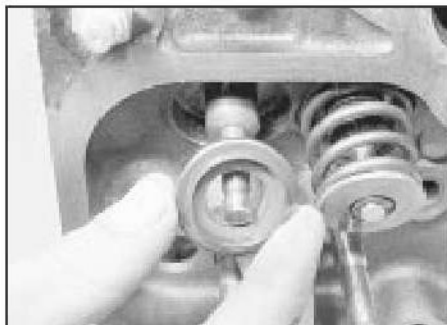
9.17 Fitting an exhaust valve rotator
