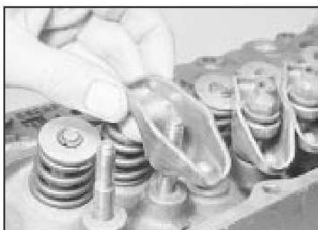
9.24a Fitting a rocker arm . . .
