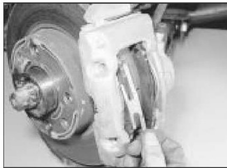
4.4a Removing an anti-rattle spring
