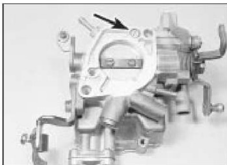
19.6 Undo the screw (arrowed) to separate the throttle valve and float chamber housings
