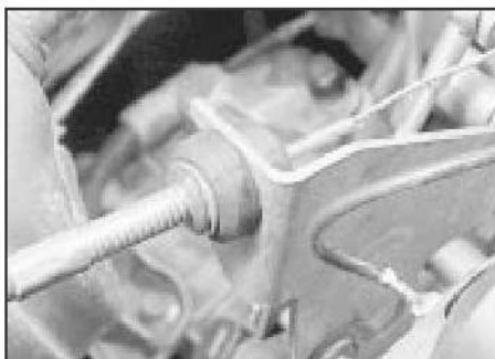
8.3 Accelerator cable bracket and bush
