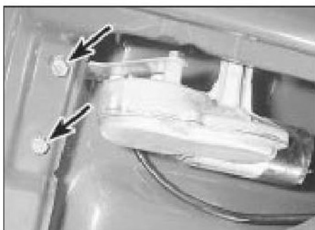
21.6 Rear wiper motor securing screws (arrowed) - tailgate-mounted motor
