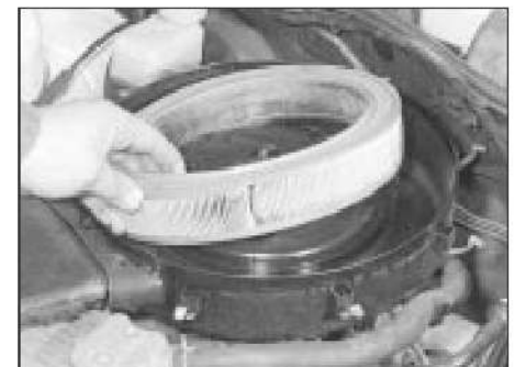
24.2b . . . and withdraw the filter element
