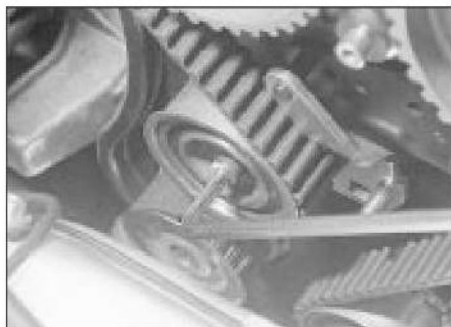
7.10 Slackening the camshaft belt tensioner screw
