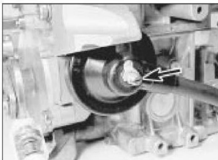
14.8a Choke valve gap adjustment screw (arrowed)
