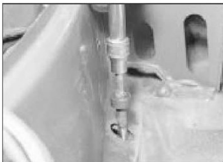
16.8 Removing a servo bracket screw
