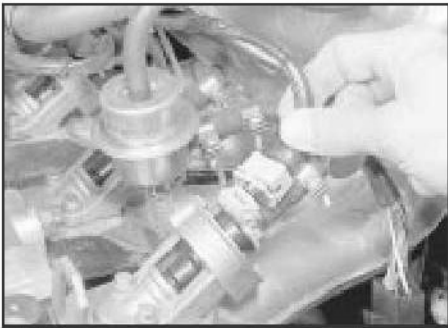
13.3b Disconnecting a fuel injector plug
