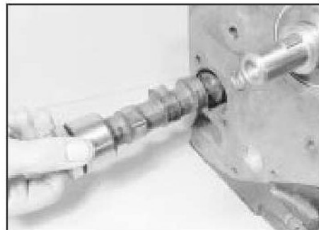
18.5 Removing the camshaft
