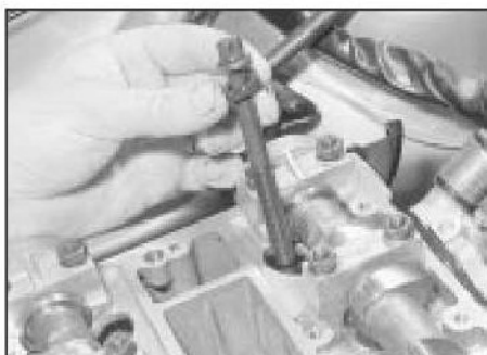
11.19b Removing a cylinder head bolt and washer
