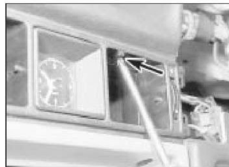
10.3 Removing a centre vent housing screw
