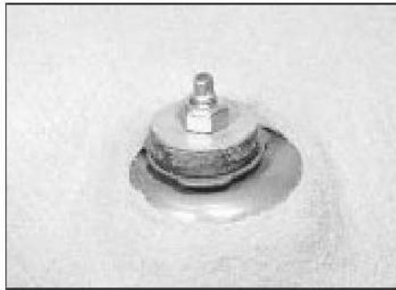
12.2 Rear shock absorber upper mounting - Hatchback
