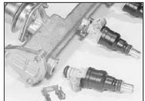
12.69b . . . and pull out the injector
