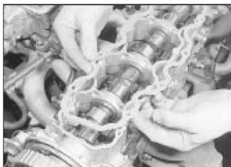
8.29a Fitting a new camshaft cover gasket
