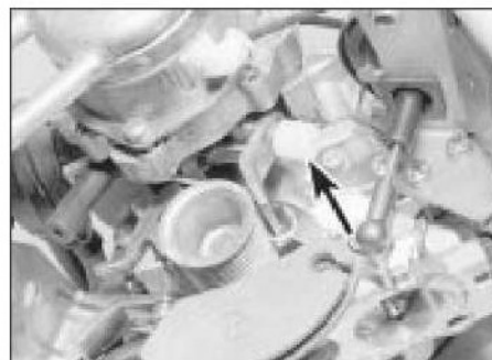
15.4 Fast idle adjustment screw under tamperproof cap (arrowed)
