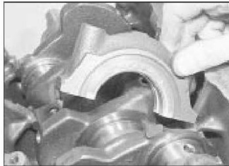
20.16a Fitting a main bearing cap
