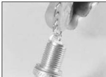
7.11 Adjusting a spark plug electrode gap using a special tool
