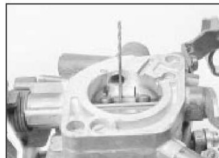
12.3 Using a drill bit to check the fast idle valve gap
