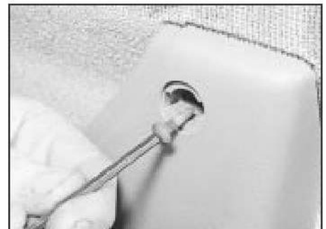
12.5b Removing a door pocket screw
