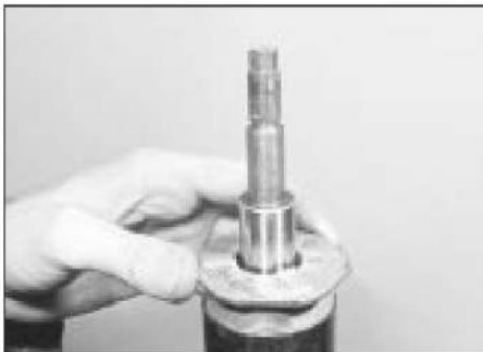
4.6b Removing the strut ring nut
