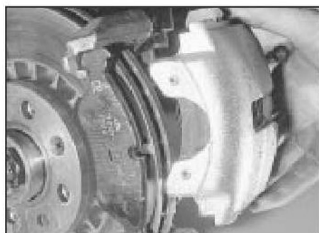
4.20 Lift the caliper off the disc ...
