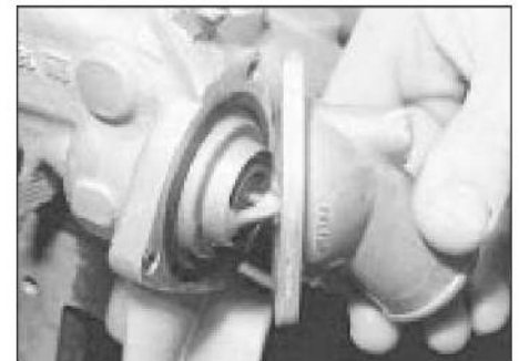
4.9a Removing the thermostat cover . . .
