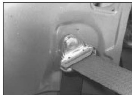
37.7b Rear seat belt upper mounting
