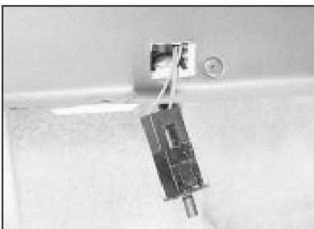
4.25a Glovebox light switch unclipped from its location
