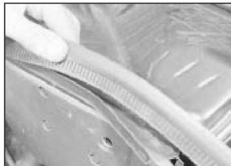
9.8a Lift the rubber seal to free the water
