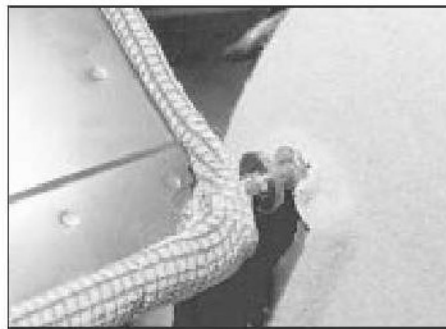
33.3b Seat pivot lifts out of hinge
