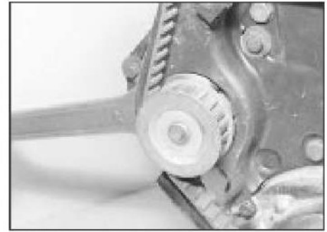
7.9 Swivelling the water pump using a spanner on the flats
