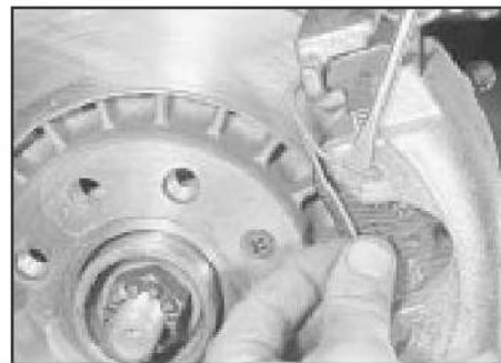
4.17 ... then lever out the spring clip
