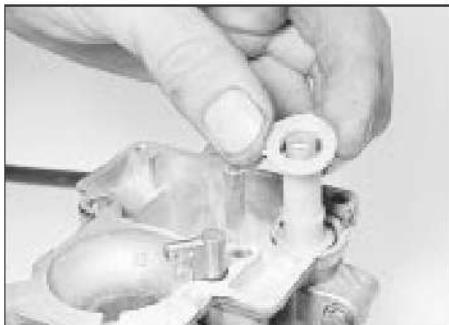
21.7a Removing the accelerator pump collar ...
