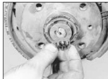
10.6b . . . the washer and the castellated nut
