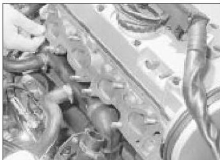
13.33 Fitting a new inlet manifold gasket
