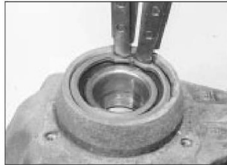
3.5b Removing a hub bearing circlip
