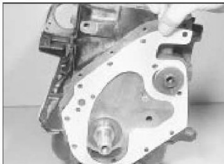
18.10 Fitting a new front plate gasket
