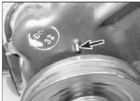
6.3 Ignition timing marks (arrowed) in alignment
