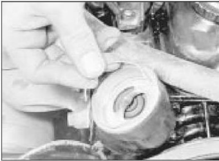
4.3a Remove the thermostat retaining snap-ring . . .
