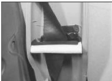
37.6b Belt feeds through guide in pillar trim
