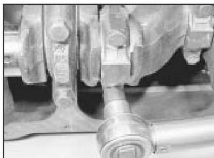
15.14b Tightening a big-end bearing cap bolt
