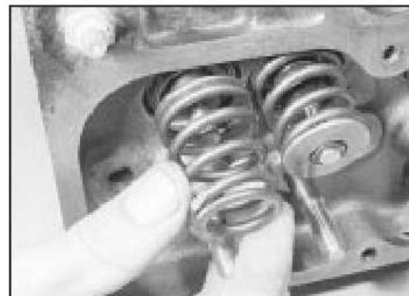
9.18a Fit the valve spring . . .
