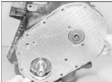
18.4b Removing the engine front plate
