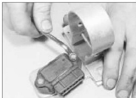
7.3 Unbolting the ignition module (1.8 litre model shown)
