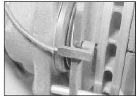
4.4b Wear warning sensor clipped to pad
