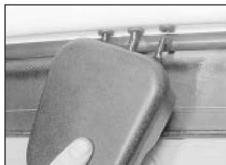
21.9 Removing the window-mounted motor
