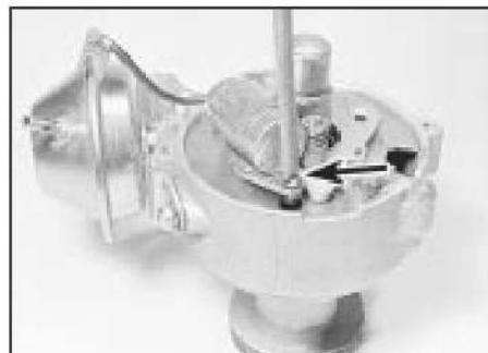
7.5 Undoing the condenser retaining screw
