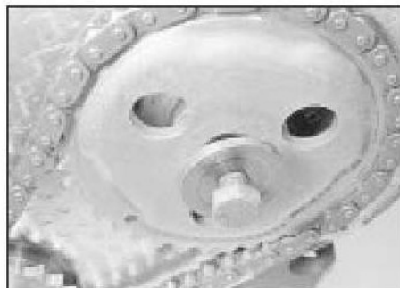
14.10 Camshaft sprocket retaining bolt and washer
