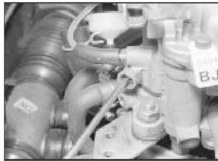
11.4c Adjusting the idle speed - Varajet carburettor
