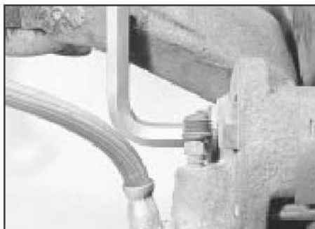
10.6b . . . then unscrew the caliper bolts . . .
