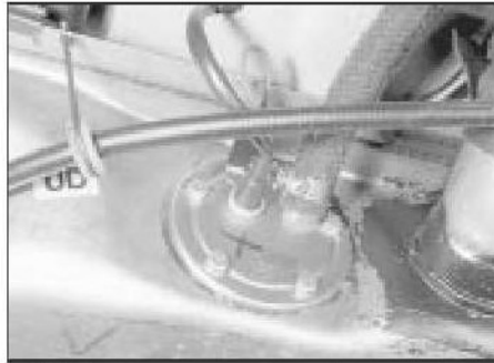
6.3 Fuel gauge sender unit secured by bolts
