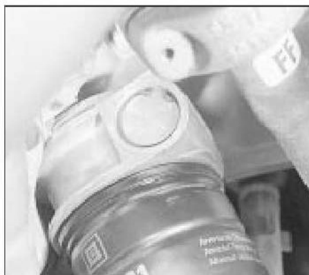
16.2 Circlip securing oil cooler thermostatic valve
