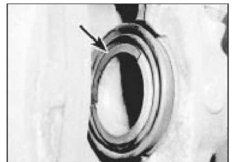
11.8 Correct position of rear caliper piston step, showing the inboard piston on the right-hand caliper. Opposite piston is the mirror image
