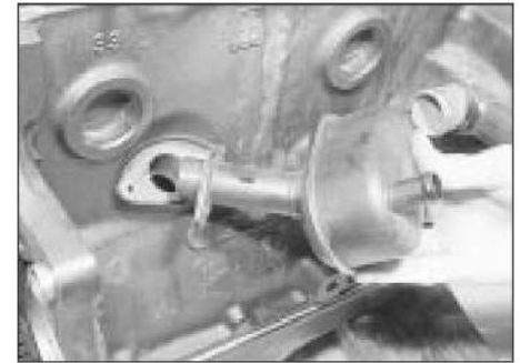
22.8 Crankcase ventilation system oil separator - 1.3 litre engine
