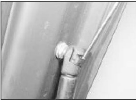
22.2 Releasing a tailgate strut spring clip
