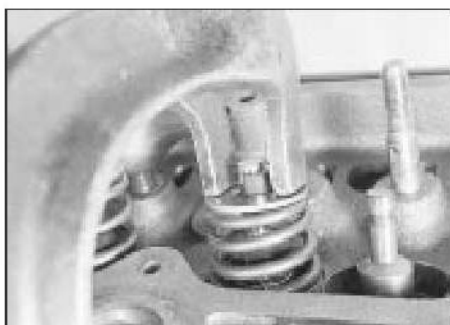
9.20 Compress the spring and fit the collets
