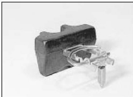
23.13 Float and needle valve
