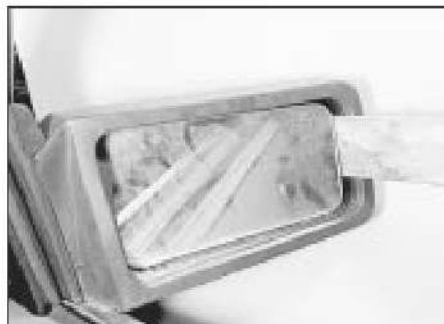
30.2a Remove the glass by levering with a wooden wedge
