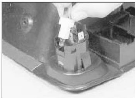
11.28 Removing a switch illumination bulb
