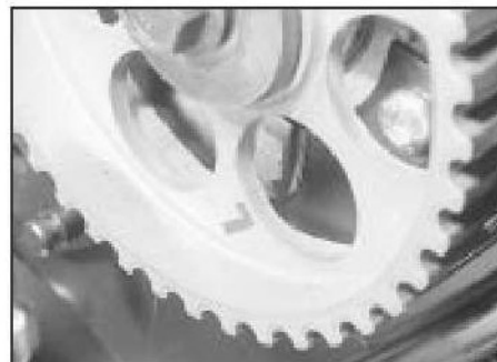
10.4 Exhaust camshaft sprocket is marked 'L'
