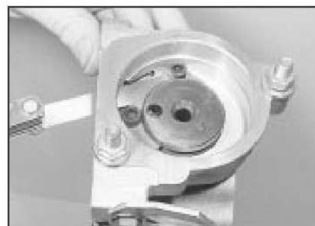
9.10 Checking the camshaft endfloat
