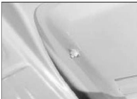
26.9 Boot lid handle retaining nut
