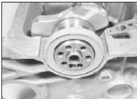
20.15a Crankshaft rear oil seal
