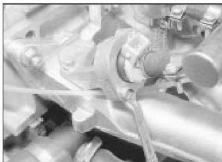
12.8 Undoing a fuel injector retaining bolt
