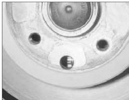
19.11a On models with rear disc brakes the handbrake shoe adjuster wheel is accessible through the hole in the disc . . .
