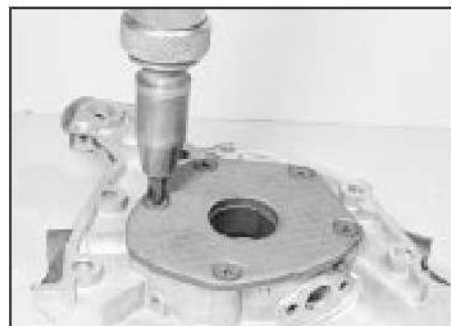
14.1 Using an impact screwdriver to undo the oil pump rear cover screws
