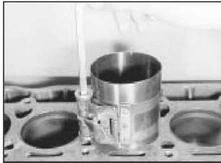
15.12 Piston ring compressor fitted
