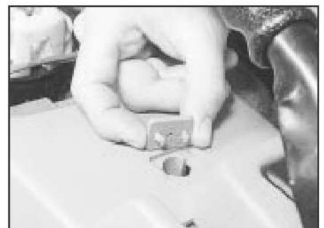
35.2a Centre console rear half screw cover
