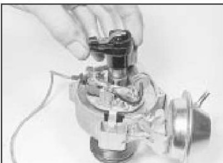
4.2 Removing the rotor arm
