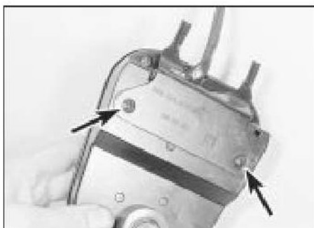
21.13a Undo the retaining screws and remove the mounting bracket . . .
