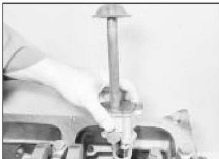
12.2b . . . and remove the oil pump
