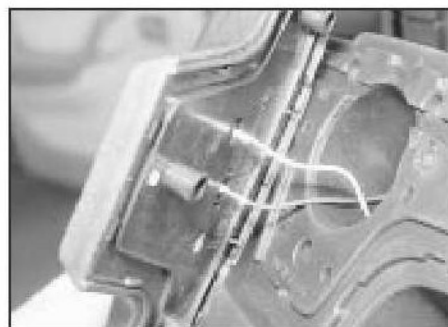
19.2 Removing the steering wheel central cap
