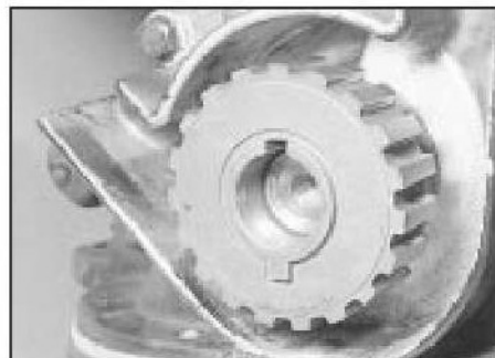
13.2a Removing the crankshaft sprocket
