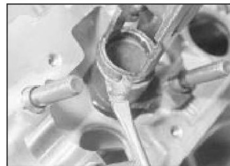
12.13 Fitting a valve collet
