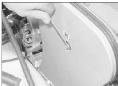
7.6a Removing a belt cover bolt ...
