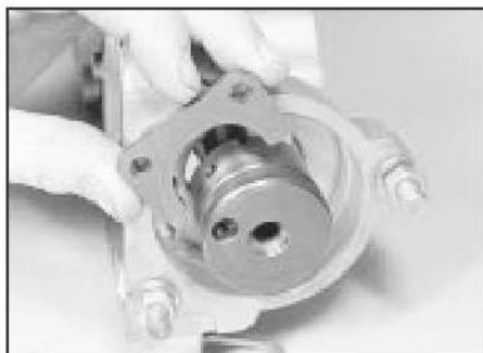
9.5b Removing the camshaft thrust plate
