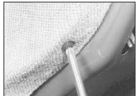
12.7 Trim securing screw on the door shut face - rear door shown
