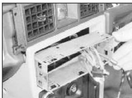
25.4 Removing the radio surround
