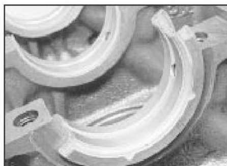
20.12 Centre main bearing shell, showing thrust flanges
