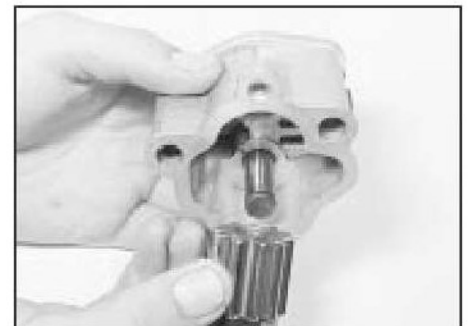
13.3b . . . and the driven gear
