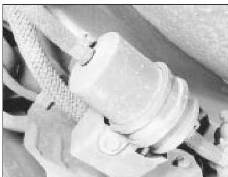
25.3 Fuel filter showing mounting and hose connections
