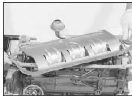
12.7a Removing the oil baffle plate. This model has two cork gaskets . . .
