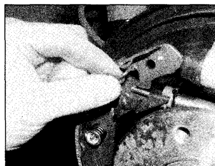
6.24b ... and secure with the retaining spring
