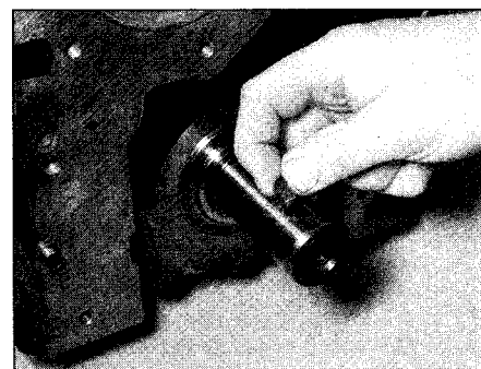
9.15b ... and remove the Woodruff key
