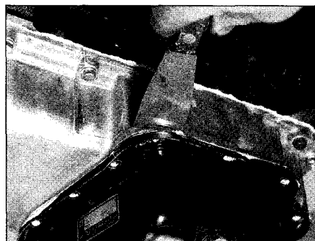
14.4 If the lower pan is stuck to the main casting, carefully ease it away using a wide-bladed scraper
