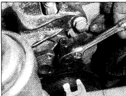
8.40 Unscrew the mounting bolts . . .
