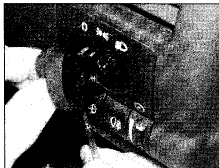
47.33 Use a small screwdriver to release the control knob from the light switch
