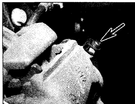
2.14 Dust cap on a bleed screw (arrowed)
