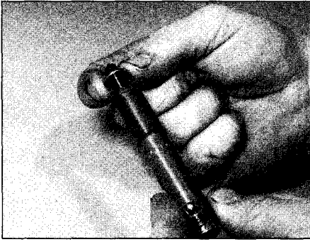
12.25a Fit a new sealing washer to the base of the nozzle . . .
