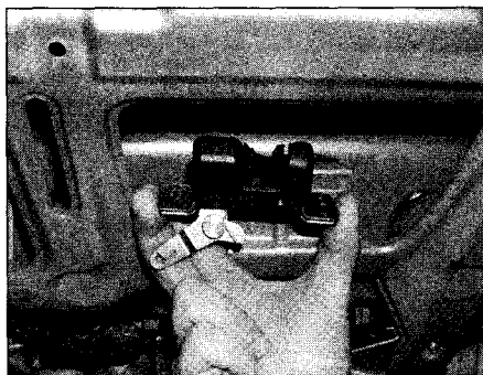
26.6d . . . and withdraw the lock from the tailgate
