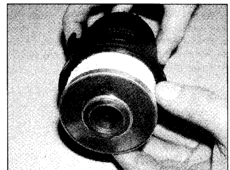
20.6c ... and filter element
