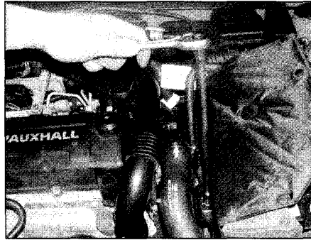
6.4a With the battery terminals disconnected, unscrew the mounting clamp bolt . . .
