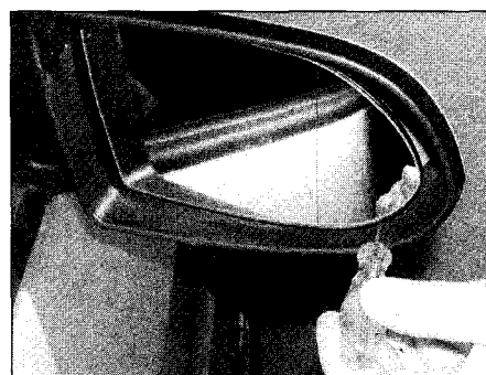
30.1 Use a screwdriver to assist removing the glass from the exterior mirror
