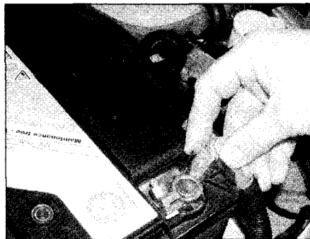
4.2 Disconnect the battery negative terminal
