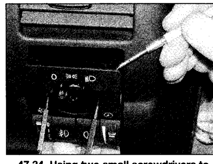
47.34 Using two small screwdrivers to release the clips when removing the light switch from the fascia
