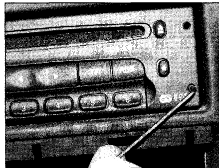
17.1 Using an Allen key to unscrew the grub screws
