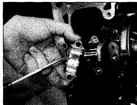
18.26 Lubricate the bearing shell with clean engine oil and then refit the bearing cap to the connecting rod . . .
