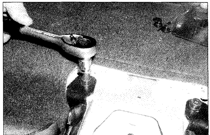
42.25 Removing the 3rd row rear seat belt stalk
