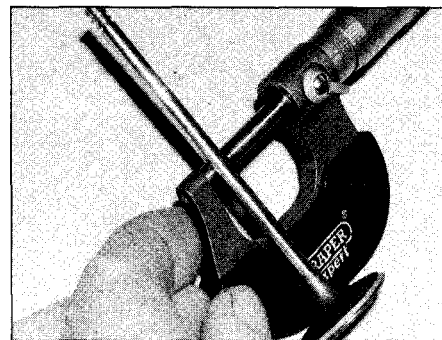
7.13 Measure the valve stem diameter using a micrometer
