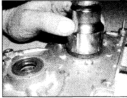
15.13 The seal fits flush with the housing
