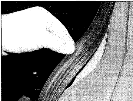
44.27 Removing the rubber weatherstrips from the body aperture
