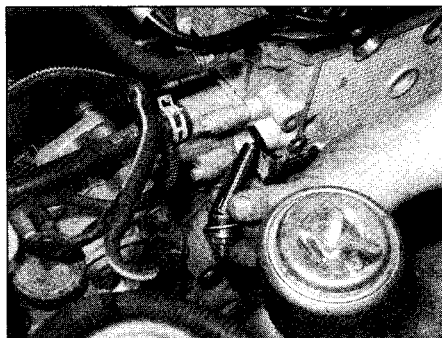
8.3b . . . and withdraw the plunger, noting which way around it is fitted
