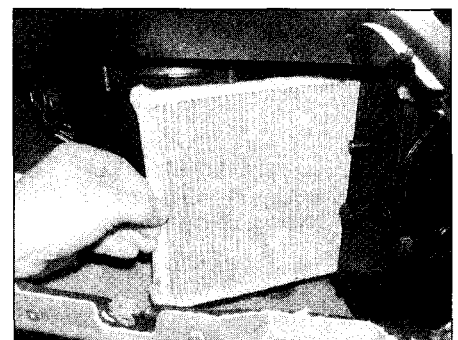
12.12 Removing the pollen filter
