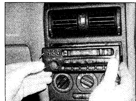
17.3b Removing the radio/cassette player - Astra
