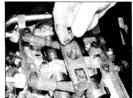
12.11 The injector clamp washer fits dished with the side facing down
