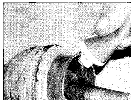
3.7 Packing the joint with grease
