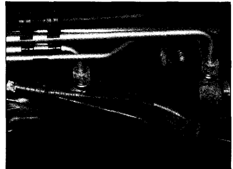
Power steering fluid may leak from the pipe connectors on the steering rack.
