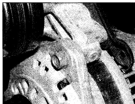
8.14a Alternator upper mounting bolt . . .
