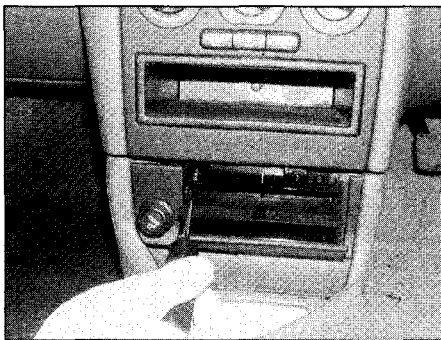
11.2a Undo the screws . . .
