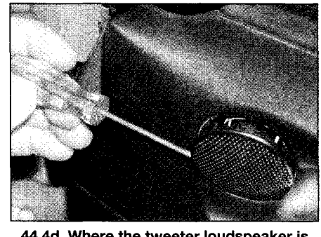
44.4d Where the tweeter loudspeaker is located in the door inner trim panel, prise it out . . .
