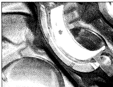
17.34 Fit the thrust washers to the No 2 main bearing with the oil grooves facing outwards
