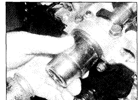
9.4 Press the oil seal into position using a tubular drift such as a socket
