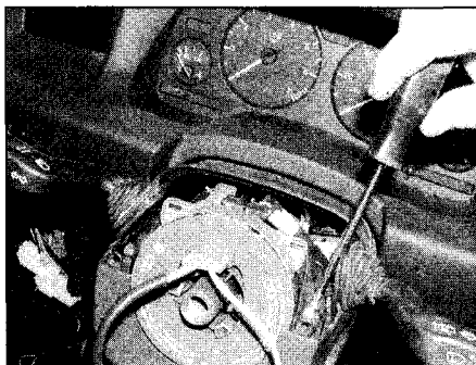
18.5a Undo the upper screws ...
