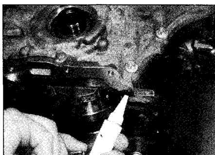
12.10a Apply a smear of sealant to the areas of the cylinder block/timing chain cover joints . . .
