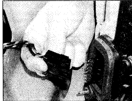
7.12 Disconnecting the wiring from the rear light cluster
