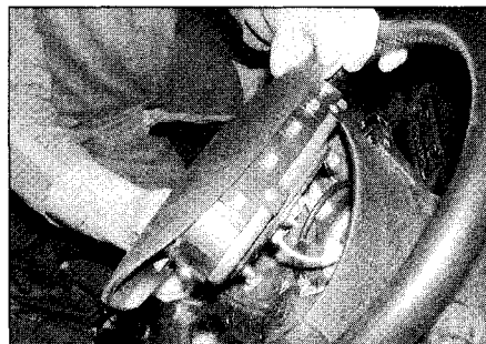
24.3b . . . and carefully lift the airbag/horn-push from the steering wheel
