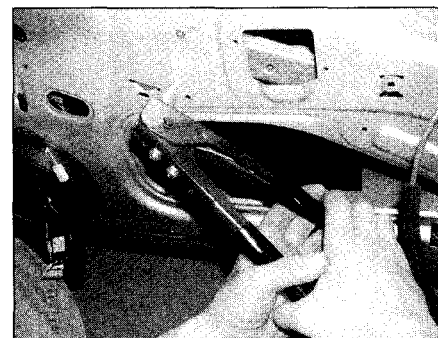
20.4 Securing the window regulator with new pop-rivets
