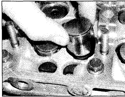
11.9 Lift out the cam followers and shims
