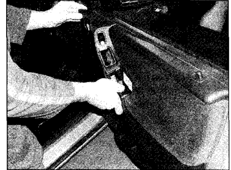
44.7b Removing the trim panel from the door
