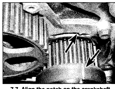
7.7 Align the notch on the crankshaft sprocket with the pointer on the oil pump cover (arrowed)
