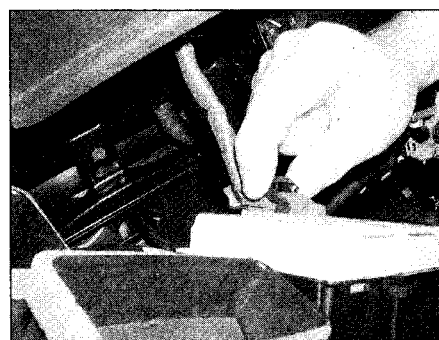
10.22 Disconnecting the wiring from the multi-function display unit – Zafira
