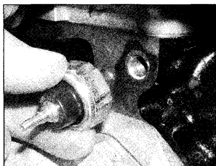
13.5 Oil pressure warning light switch – 1.7 litre DOHC engines
