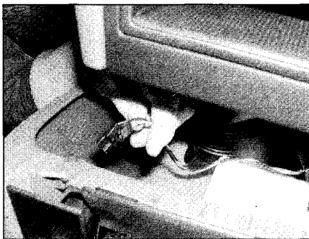
11.2b . . . remove the ashtray and disconnect the wiring
