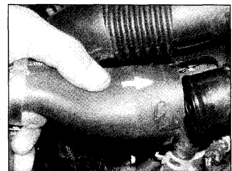
6.6 Disconnecting the air inlet duct from the air inlet plenum intermediate pipe
