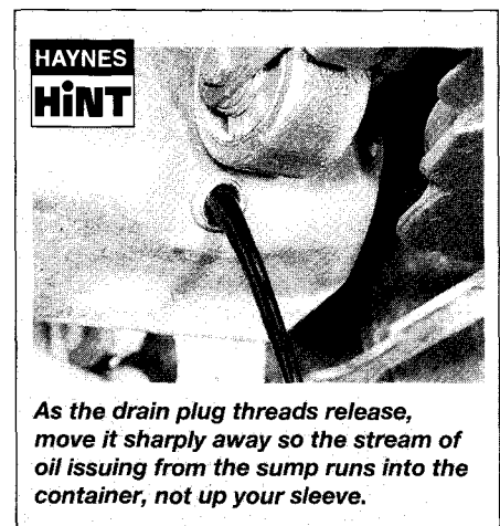
4.5 Sump drain plug – 1.7 litre engine
