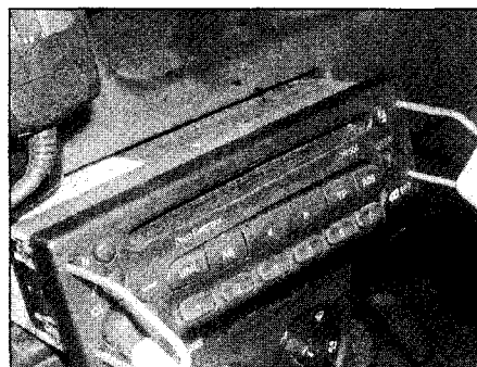
17.2 Insert the two DIN removal tools . . .
