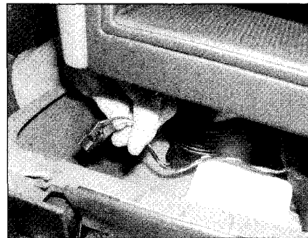
45.8e ... and disconnecting the wiring for the cigarette lighter
