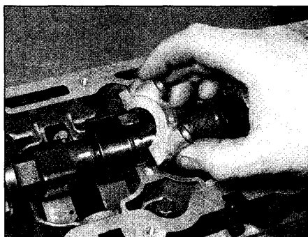
10.25 Refit the camshaft bearing caps using the identification markings to ensure each is correctly positioned
