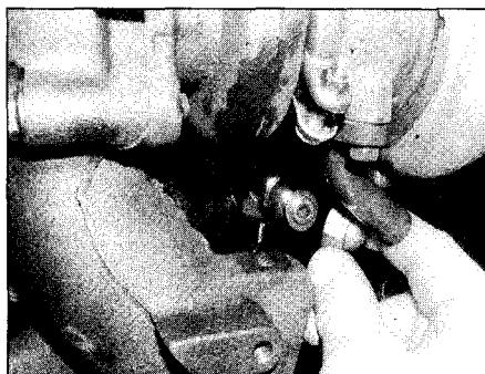
16.26 Remove the oil feed pipe from the cylinder block
