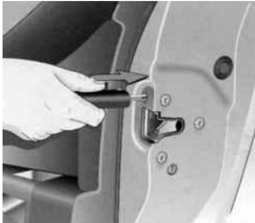
Fig. 1.19. Removal of the central locking device malfunction
