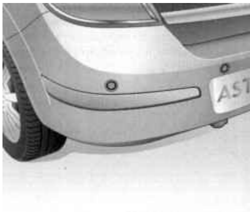
Fig. 1.48. Sensors "parking pilot"
