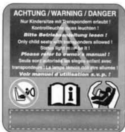
Fig. 1.57. Label indicating that the system is installed in a car seat recognition of employment
