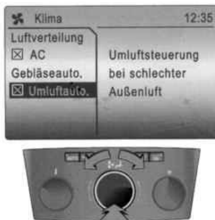
Fig. 1.136. Selecting the automatic air circulation
