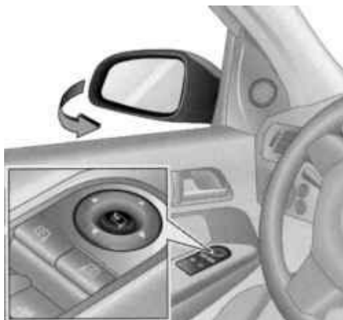
Fig. 1.149 . To fold the automatic rear-view mirror
