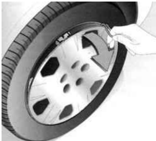
Fig. 1.255. Removing wheel cap
