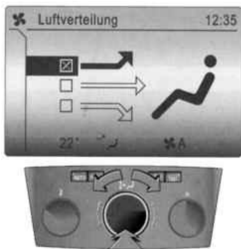
Fig. 1.133. Vlyuchenie mode of air distribution
