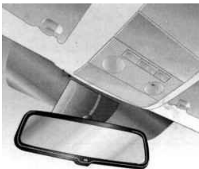
Fig. 1.144. Automatic anti-dazzle interior mirror
