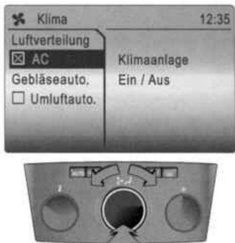
Fig. 1.132. Mode on and off air conditioning compressors
