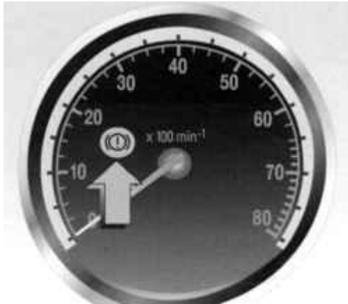
Fig. 1.37. Control lamp sensors malfunction of the braking system / indicator applying the parking brake
