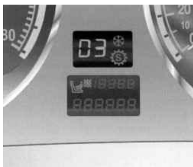
Fig. 1.223. Display mode D automatic gearbox for the Information Display
