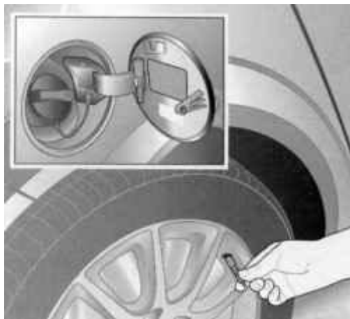
Fig. 1.238. Location puller lid valves
