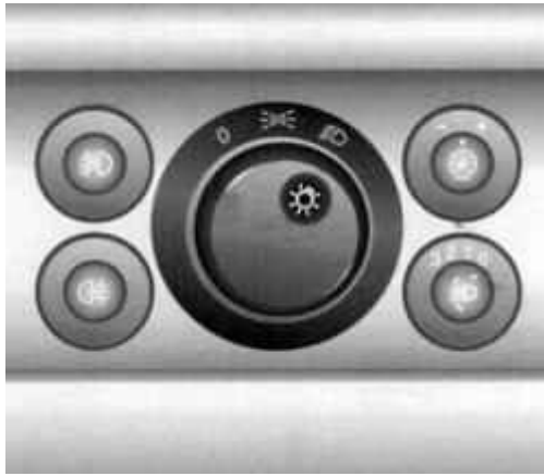
Fig. 1.44. Control panel exterior lighting
