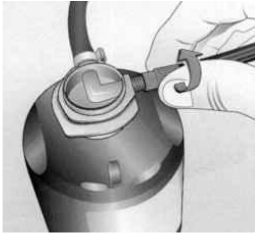
Fig. 1.268. Installation of air compressor hose
