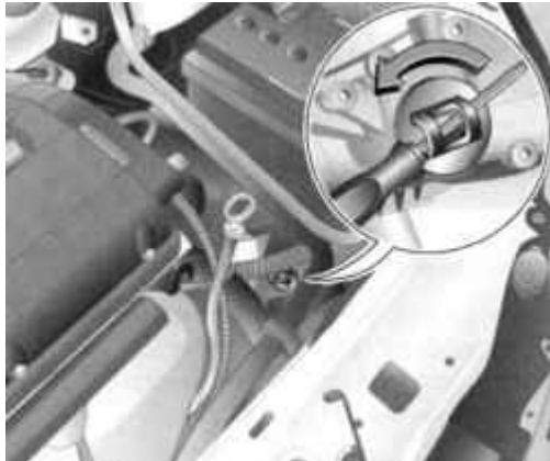
Fig. 1.41. Removing the automatic transmission Easytronic
