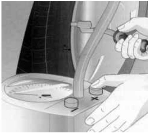
Fig. 1.240. Screwdriving valve cover special key
