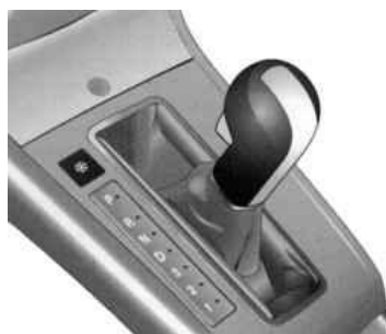
Fig. 1.222. Lever switch mode automatic transmission
