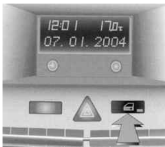
Fig. 1.17. Key unlocking and locking the car doors from inside
