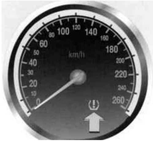
Fig. 1.60. Alarm monitoring system pressure drop and the current tire pressure
