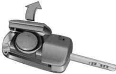
Fig. 1.13. Replacing the battery of the remote control
