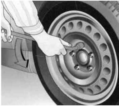
Fig. 1.257. Loosening wheel bolts
