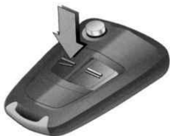
Fig. 1.27. Deactivating the partial deactivation of anti-theft system
