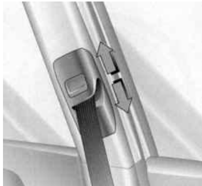
Fig. 1.209. Adjusting the height of the upper guide element of the front and rear seat belt
