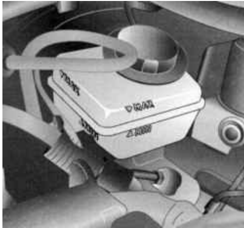
Fig. 6.12. Tank for brake fluid
