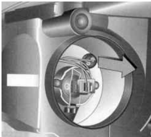
Fig. 1.287. Removing the lamp holder
