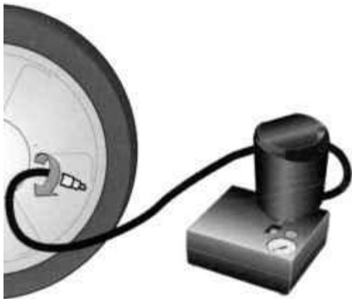
Fig. 1.269. Binding the hose to the valve to inflate the tires
