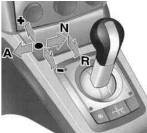
Fig. 1.218. Scheme switching modes of transmission Easytronic
