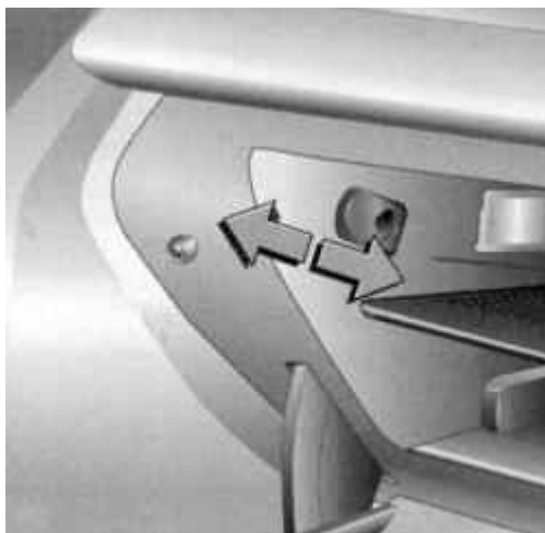
Fig. 1.138 . Enabling and disabling airflow to the front glove compartment
