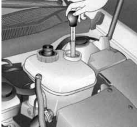
Fig. 1.275. Check the concentration of antifreeze
