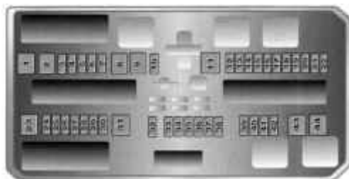
Fig. 1.315 . Fuse block, located in the trunk of a car
