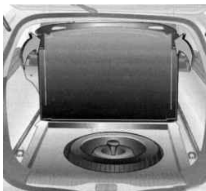
Fig. 1.252. Removing the spare wheel
