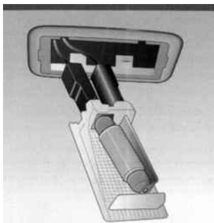
Fig. 1.312 . Removing the lamp
