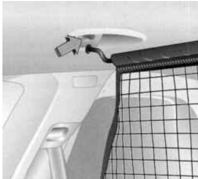
Fig. 1.194. Install barrier lattice
