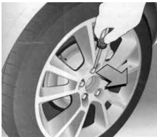
Fig. 1,256. Removing plugs wheel bolts
