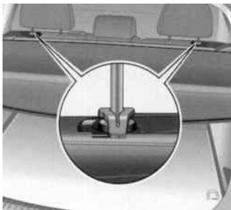
Fig. 1.192 . Closing the gap between the hood and trunk of the rear seat backs
