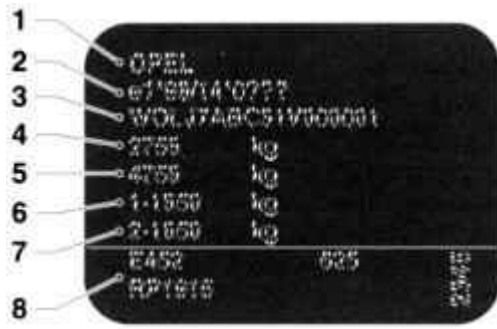
Fig. 1.2. Data on the type label: 1 - the country of manufacture; 2 - permit number; 3 - Vehicle identification number 4 - a permissible total weight, 5 - a permissible total weight of the trailer, 6 - the maximum permissible load on the front axle, 7 - maximum permissible load on rear axle, 8 - Individual vehicle data or data specific to the country
