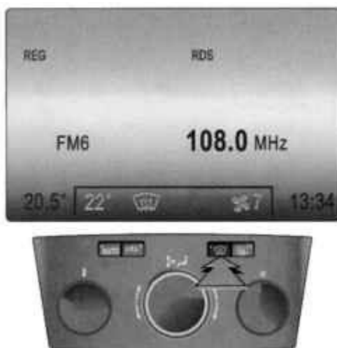
Fig. 1.131. Shutting down the regime remove moisture and frost from the glass
