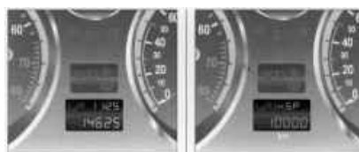
Fig. 1.71. Indication of the switching modes odometer
