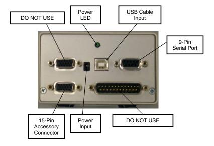
Ensure that you do not use the upper 15-pin accessory connector or the 25-pin ADC connector on the back of the ADC1000-USB-S. Using these ports may result in invalid data being returned to your spectrometer.
