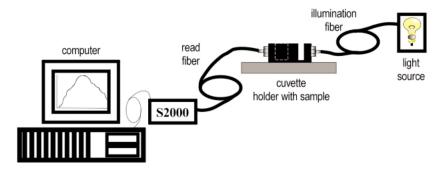
A typical configuration for a transmission experiment.
