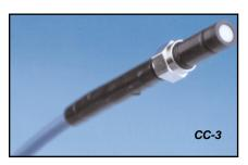
♦ The FL-400 FLAME-RESISTANT FIBER PROBE is a heat-resistant fiber optic probe that couples to Ocean Optics miniature fiber optic spectrometers to measure *in situ* emission spectra of samples such as dissolved metals and high-temperature plasmas. The FL-400 is a high-temperature 400 μm gold-jacketed UV-VIS optical fiber in an 8" long nickel sleeve. It can operate in environments up to 750° C. The probe accepts a standard wire loop for emission measurements of dissolved metals.
