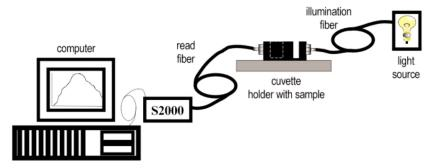
A typical configuration for an absorbance experiment.
