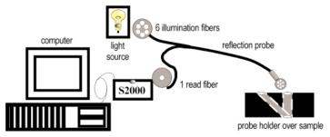
A typical configuration for a reflection experiment.
