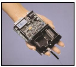
An S2000 Miniature Fiber Optic Spectrometer without its housing.
