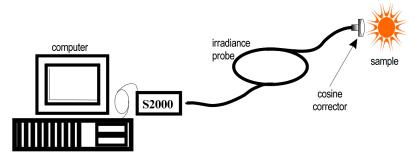
A typical configuration for an irradiance experiment.
