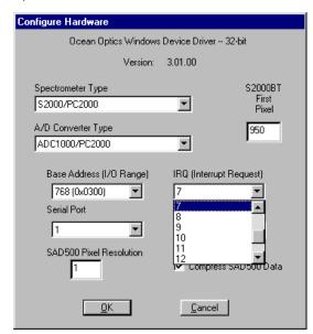
• Compress SAD500 Data. Enable this function to minimize the amount of data transferred over the RS-232 connection. Transmission of spectral data over the serial port is a relatively slow process. Enabling this function insures that every scan transmitted by the SAD500 will be compressed, greatly increasing the data transfer speed of the SAD500. (This entry is for SAD500 A/D converters.)
