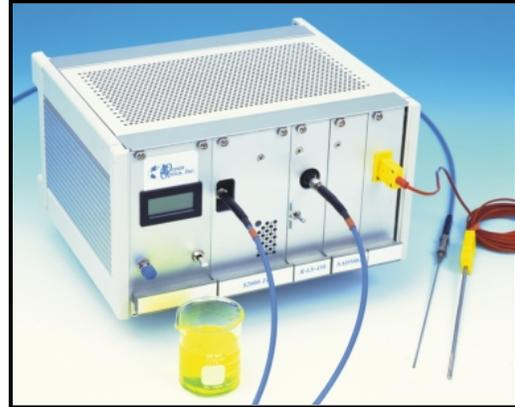
*A complete FOXY system in one box: temperature regulated spectrometer, LS-450 Blue LED, FOXY-TK1 Thermocouple and a FOXY-R probe*
