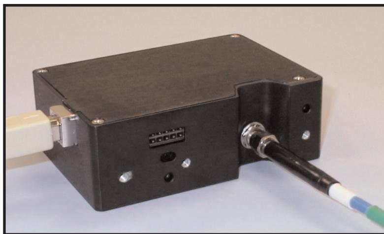
*An USB2000 Miniature Fiber Optic Spectrometer with USB cable (at left) and optical fiber (at right).*
