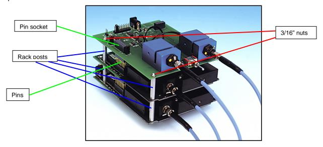
Sample Ocean Optics rack-mount system illustrating rack post assembly. In this illustration, the R-LS-450 is shown instead of the R-LS-1.
