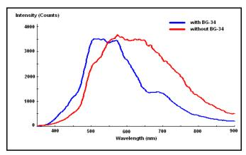
Comparison of typical LS-1 Scope mode signal with and without BG-34 filter
