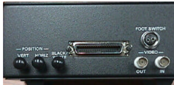
Figure 3-4 Remote Control Panel Connections.
