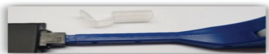
Cleaning tool with adaptor removed and the tip in a through adaptor for cleaning internal connector or a fiber port requiring cleaning
