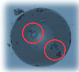
Chips are present on the end face of the connector
