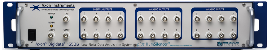
Figure 3-1: Front panel of the Digidata 1550B digitizer.
