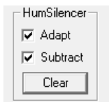
Figure 3-4: The HumSilencer system Real Time Controls panel items in active learning mode and actively canceling noise.
