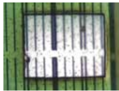
Flaking of polyimide membrane
