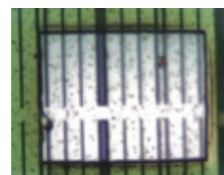
Flaking of polyimide membrane
