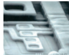
SEM photograph of IC surface after removing upper layer
