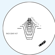
No.12AAG849 (MF D)*2 Involute gear reference rack m = 0.1 to 1.0, pressure angle: 14.5° Line width: 7µm
