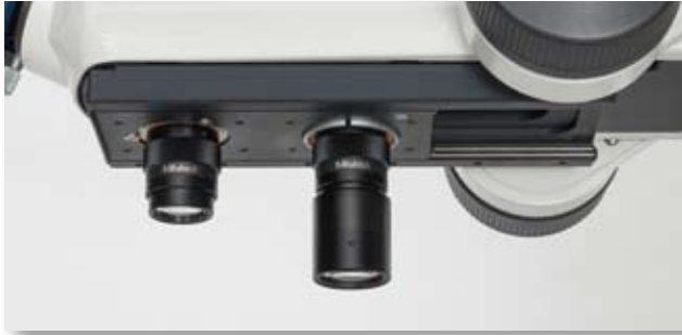
Sliding nosepiece with two objectives mounted.
