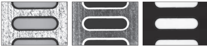
Surface illumination Programmable ring light illumination Contour illumination
