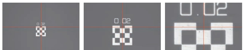
Turret 1X Field of view: 6.27×4.70 mm Turret 2X Field of view: 3.13×2.35 mm Turret 6X Field of view: 1.04×0.78 mm
