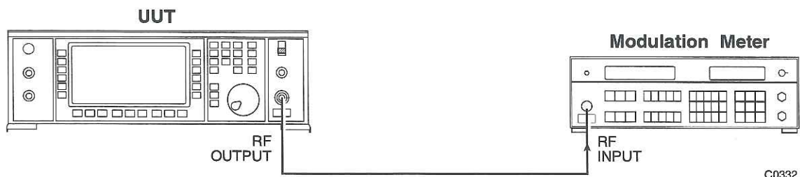
Fig. 5-2-8 Equipment configuration for the AM tests
