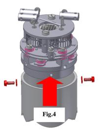
It is worthwhile at this stage to see if the source requires any attention, especially if the filament(s) have broken because of an over pressure situation in your vacuum system.
