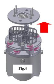
It is worthwhile at this stage to see if the source requires any attention, especially if the filament(s) have broken because of an over pressure situation in your vacuum system.
