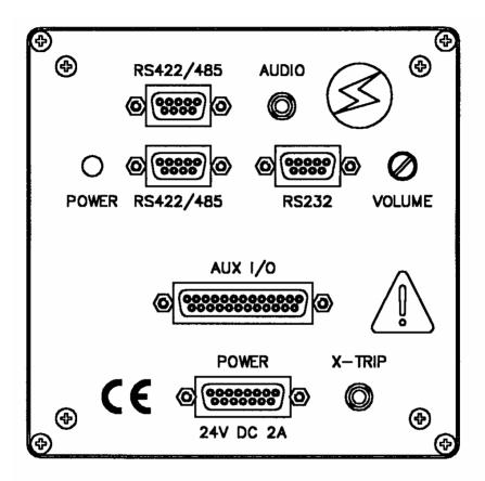
Figure 1 Rear panel arrangement
