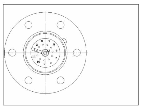
Figure 2 Analyser pin configuration
