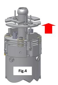
It is worthwhile at this stage to see if the source requires any attention, especially if the filament(s) have broken because of an over pressure situation in your vacuum system.
