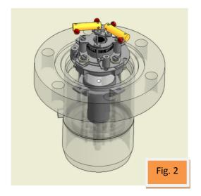
It is worthwhile at this stage to see if the source requires any attention, especially if the filament(s) have broken because of an over pressure situation in your vacuum system.
