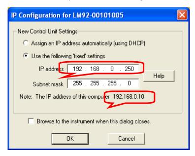
In the above case communication between the host PC and the instrument is possible, though Device Manager will recommend you change the instruments IP address to another, not ending in .250. This is to avoid potential problems when installing more than one instrument.
