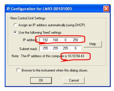
In this example, the host PC will not be able to communicate with the instrument while the two IP addresses are in different ranges.
