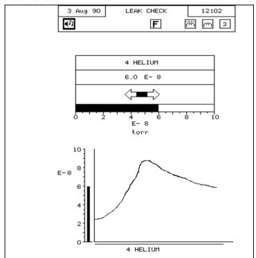
Leak checking is one of the fundamentals of vacuum system maintenance and it is a function expected of any modern day RGA. Quadrupoles have simplified the process of leak checking.
