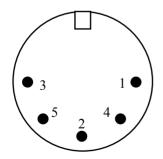
The Chart Recorder connector is a  $180^{\circ}$  5 pin DIN socket. The above is a view looking at the rear of the Vacscan instrument.
