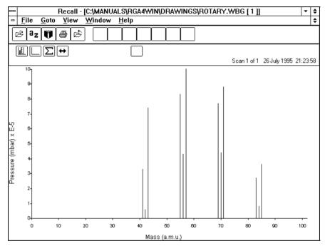
Figure 8 Rotary pump oil
