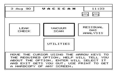
Press the **RIGHT ARROW** key once to move the cursor box (which always appears over the default mode - VACUUM SCAN) to RESIDUAL GAS ANALYSIS and select this mode by pressing the **ENTER** key. The following display will appear:-
