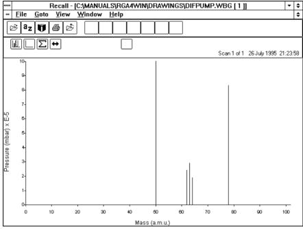
Figure 9 Polyphenylether diffusion pump oil
