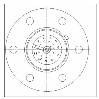
Figure 2 Analyser pin configuration
