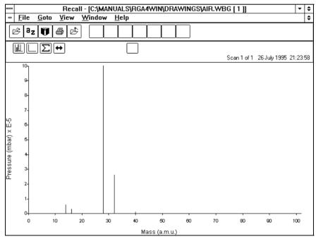
Figure 6 Air leak
