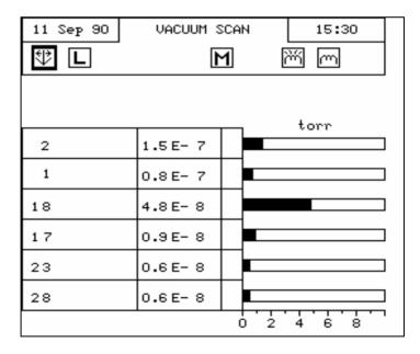
Vacuum scan is a fully automated vacuum analysis program, which, once instigated, can be left on its own. It will scan the vacuum system for the six largest peaks, display them in descending order of intensity then present you
