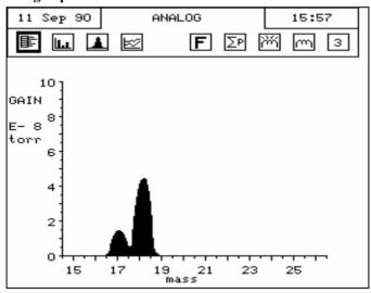
This is not an analytical mode. It is provided more as a means of monitoring the general condition of the quadrupole analyser. The conventional analogue display that is produced by this mode can provide engineers with information to help in assessing the operational condition of the instrument. It does provide an output of a type many of us are more familiar with and reminds us that the Vacscan is a quadrupole at heart.
