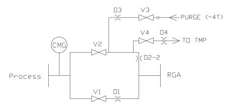
Fig.2: 4-Valve, Fast-Response "LPCVD" Configuration
