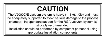
Note that care must be taken to support the weight of the V2000C/E assembly (approx. 18kg, =40lb) at the tool. Most process tools have aluminium chamber walls with fittings that will not support this weight and torque, directly.
