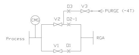
Fig.1: 3-Valve "Etch" Configuration
