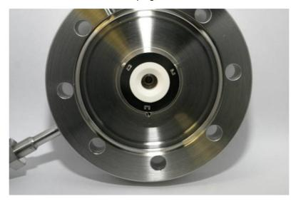
In order to use the orifice disk insertion and removal tools, this coupling must be removed from the inlet flange.
