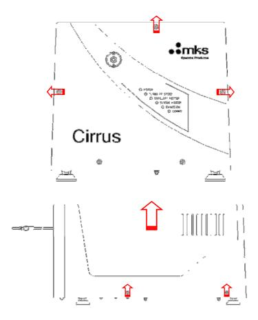
Remove the two Allen head bolts from either side of the outer cover.
