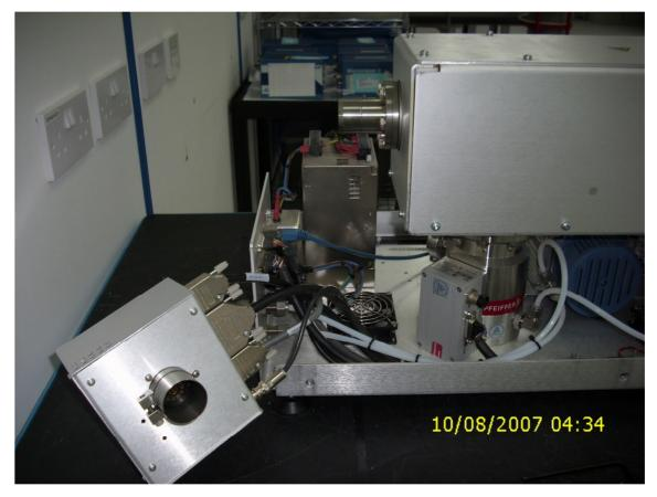
3. Make a note of the orientation of the analyser with respect to the vacuum chamber. Use the locking pip on the analyser flange as a reference (it will usually be in the 12 o'clock position).
