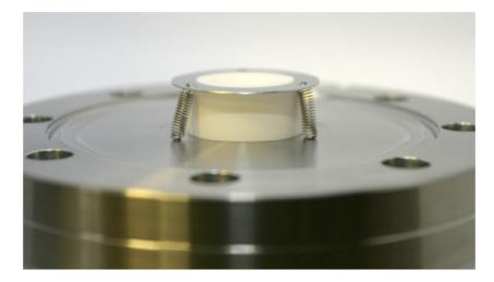
5. Clean all handled parts with a suitable solvent and re-fit the Inlet Flange to the chamber using a new copper gasket, by firstly sliding the bypass connection through the oven wall and then carefully locating the Ceramic Coupling over the PVD ion-source of the quadrupole.
