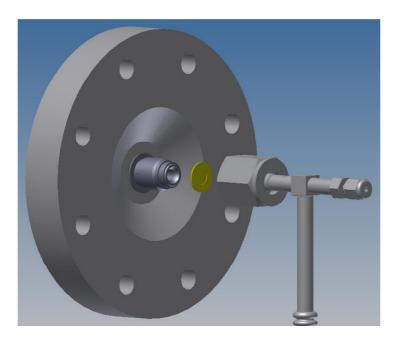
To replace the disk, follow the steps on removing the outer cover detailed in the preceeding section to allow access to the inlet flange.
