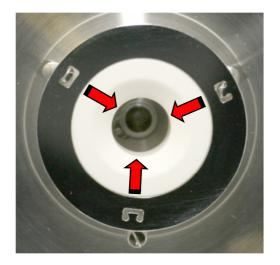
8. Remove the retaining plate and ceramic coupling from the inlet flange.
