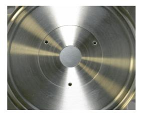
Without disturbing the new Orifice Disk, carefully re-fit the tool guide to the inlet flange. Once the guide is secured, check again that the new Orifice Disk is lying squarely in the tapered hole. If not, it must be re-positioned. Use the Insertion Tool to push the Orifice Disk into the tapered hole. Some resistance will be felt as the disk seats into position. Push the insertion tool fully into the tool guide.
