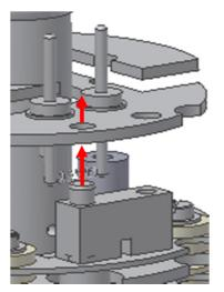
2. Loosely re-fit the four M2 x4 pan head screws through the filament plates.
