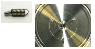
Once all three springs have been removed we can proceed to remove the orifice disk using the removal tool.
