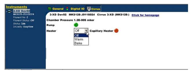
The multiplier detector will be unavailable during baking and for a period afterwards while the system cools down.
