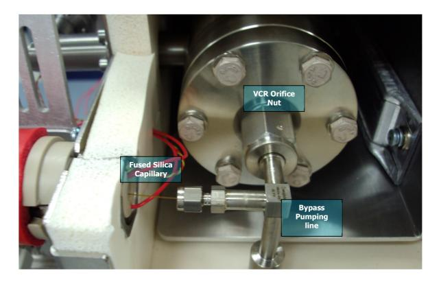
Illustration 10. Top Rear View of Cirrus 3-XD, with fused silica capillary and VCR Orifice connection. The example shown is for the rack mounted Cirrus 3-XD, the desktop version has the capillary entering from the other side.
