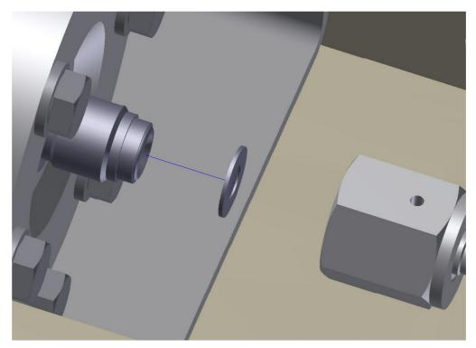
Illustration 13. To replace the disk, follow the steps on removing the outer cover detailed in the preceeding section to allow access to the inlet flange.
