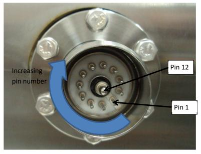
Illustration 18. Pin 1 is recognised by the track connecting it to earth, the pin number increases in the clockwise direction, pin 12 is the center pin.
