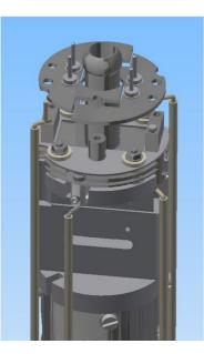
Illustration 22. Carefully remove filament plates
