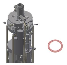
Illustration 26. Remove screw and withdraw wire
