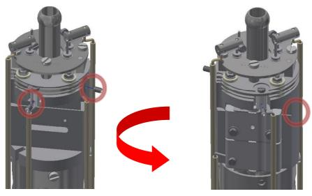
Illustration 24&25.Remove grub screws and withdraw wires
