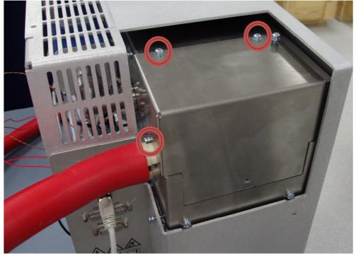
Illustration 9. To remove oven entrance hatch, loosen or remove three screws and lift off cover, to gain access to change the fused silica and VCR orifice
