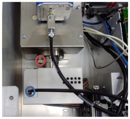
Illustration 16. Unplug the coaxial cable indicated with the blue circle and loosen the bolt in the red circle with a 4mm allen key untill the collar moves freely. Pull the box connected to the analyser away towards the front of the instrument, place it clear as shown below.
