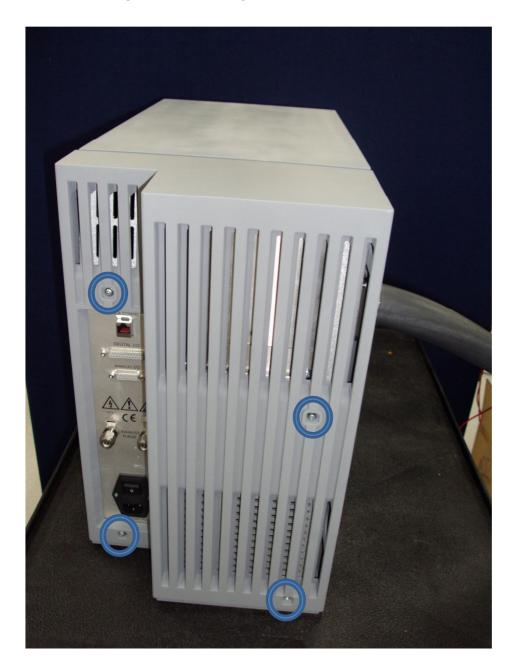
Illustration 3. To access the rear of the instrument, required for changing the capillary and orifice disk, the rear panel must be removed. This is done by removing the four screws and pulling the panel backwards until clear of the instrument.
