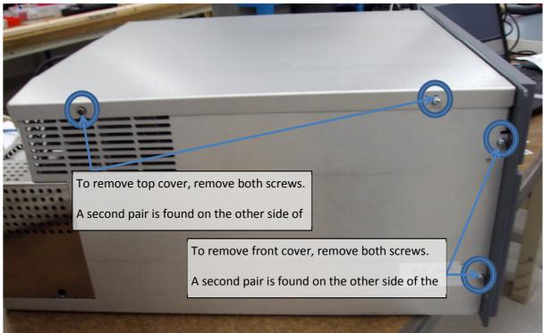
Illustration 6. Removal of the front and top panel is required to access the mass filter for source maintenance.
