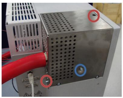
Illustration 5. To access the rear of the instrument, required for changing the capillary and orifice disk, a small rear cover must be removed.
