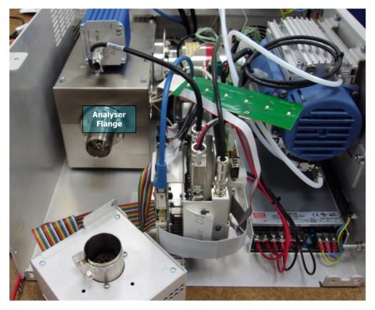
Illustration 17. Cirrus 3-XD with LED pcb and RF/electrometer unit de-mounted.
