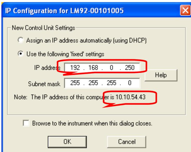
In this example, the host PC will not be able to communicate with the instrument while the two IP addresses are in different ranges.
