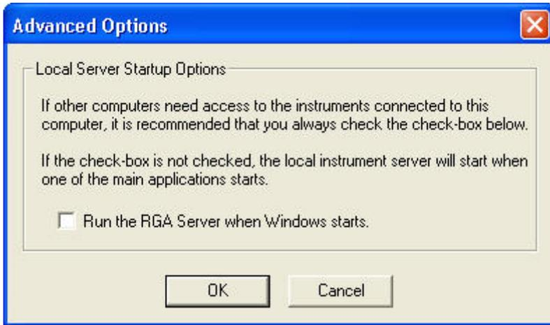
If network access for the local instrument is required, check the **Run the RGA Server when Windows starts** option. This will start the server program whenever Windows starts. If the option is not checked then the server program will only start when one of the MKS RGA Applications such as Process Eye Professional starts
