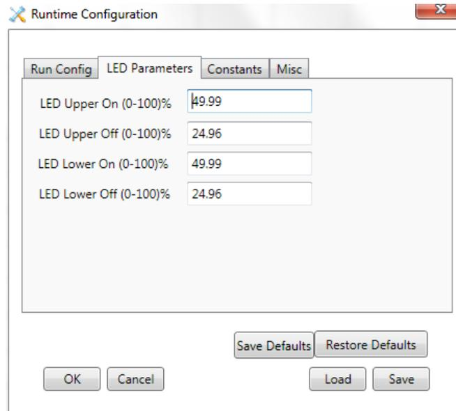
The On and Off powers for the LEDs are set here. When values are entered, the software will set the closest digital value for the chosen power, when re-opening the dialog box this will show a value that is the closest digital fit to the chosen power (a 12 bit digital to analog convertor is used).
