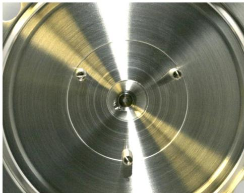
Once all three springs have been removed we can proceed to remove the orifice disk using the removal tool.
