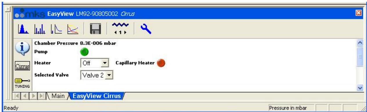
The chamber pressure is the value obtained from the internal gauge situated close to the turbo pump. Click on an indicator to change its state. If you have a multi-valve inlet you can change the active inlet using the drop-down list. The list always shows the currently active inlet.
