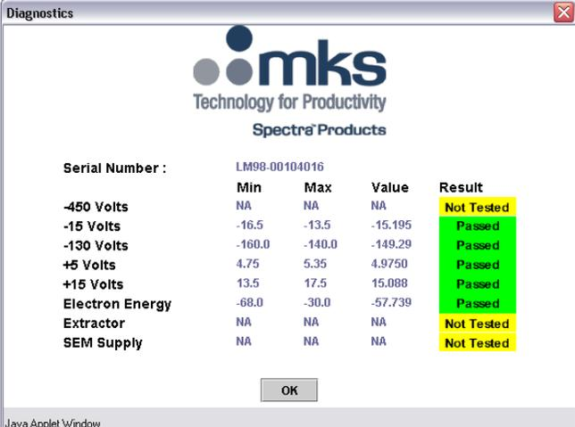
The screenshot shows a window titled "Diagnostics" with the MKS logo and "Technology for Productivity Spectra Products" text. Below this, the "Serial Number" is listed as "LM98-00104016". A table displays test results for several parameters, with columns for "Min", "Max", "Value", and "Result". The results are color-coded: yellow for "Not Tested" and green for "Passed". An "OK" button is located at the bottom of the table area. The window footer indicates it is a "Java Applet Window".
