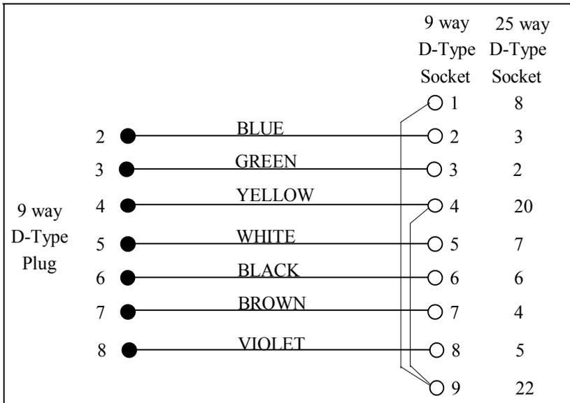
Figure 5 RS232 cable connections
