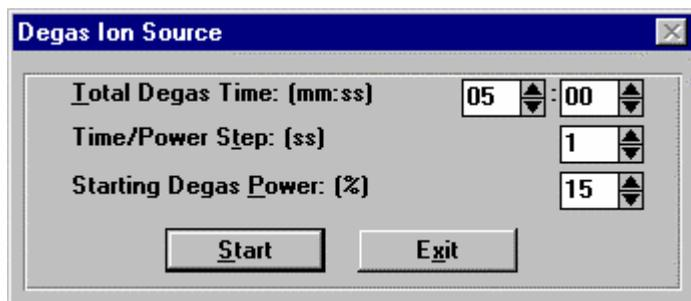
To enter the Degas Setup *dialog box* select RGA | Degas from the *menu bar* or *click* on the Degas button in the Mode Select screen. Before the *dialog box* is displayed, if the filaments are off, you will be given the option of turning on a filament before you proceed.
