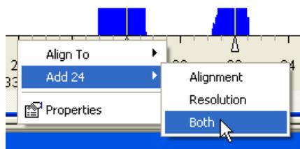
In this example we are adding both an Alignment and Resolution points at mass 24.
