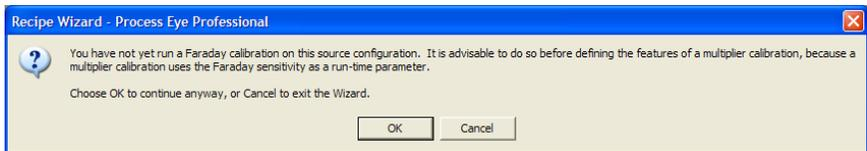
This simply states that whilst the multiplier will be calibrated to the current Faraday measurements, resulting multiplier measurements will be inaccurate as "real" measurements in the same way as the Faraday measurements are. If you are happy with this, click **<OK>**.
