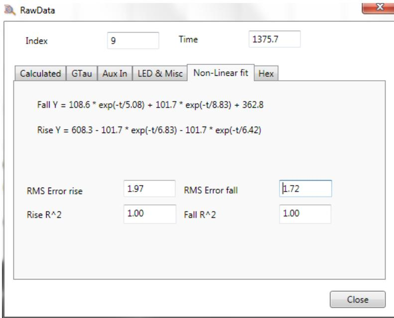
The Non-Linear fit data is only populated if the Configure dialog's Misc./Post Fit type is set to Single or Double exponential. The linear domain rise and fall equations are displayed along with the RMS error and R<sup>2</sup> correlation coefficients.
