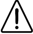
The Exclamation Mark (ISO 3864, No.B.3.1) on the rear panel relates to Mains input and fuses specifications. See Section 2.2.2 Electrical..
