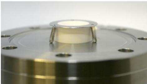
Clean all handled parts with a suitable solvent and re-fit the Inlet Flange to the chamber using a new copper gasket, by firstly sliding the bypass connection through the oven wall and then carefully locating the Ceramic Coupling over the PVD ion-source of the quadrupole.
