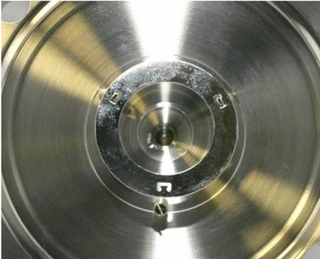
From the side without a spring fitted, slide the Ceramic Coupling under the Retaining Ring, paying attention to the couplings orientation, which should be with the shouldered face uppermost.
