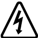
The Electric Shock (ISO 3864, No.B.3.6) symbol placed on the top cover refers to the risk of Electric shock from Hazardous voltages if the covers are removed.
