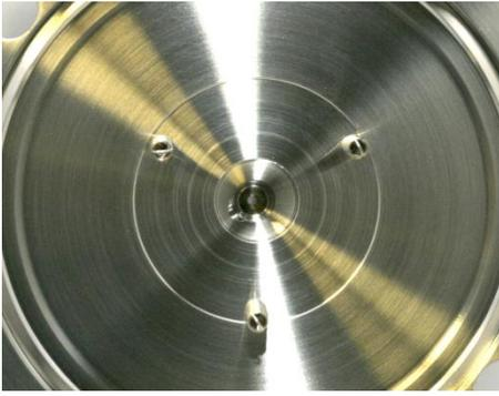
Secure the Retaining Ring by using two of the three springs.
