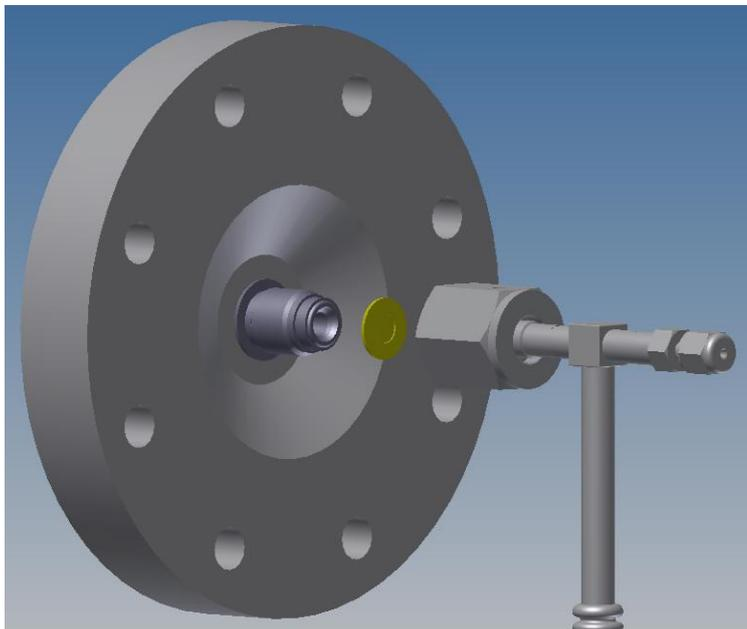
To replace the disk, loosen the VCR fitting using a  $\frac{3}{4}$ " spanner, the disk is fitted into a formed holder which is clipped onto the machined face of the inlet flange. Remove the old disk and replace with the new part, refit the holder to the inlet flange and retighten the VCR fitting.
