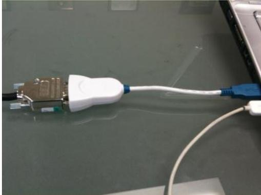
2. Connect Serial connect to GLM 2000 (shown above)
