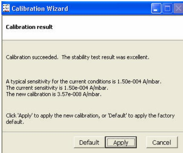
The stability of the calibration is calculated as a percentage, based on the following formulas:
