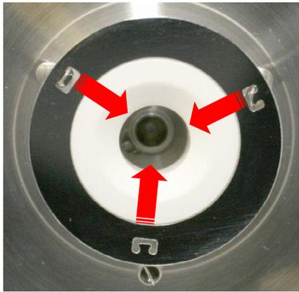
Remove the ceramic coupling retaining ring by easing the retaining springs from their fitting points.
