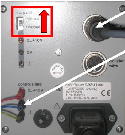
Move the Set Point switch to the INTERNAL position.
