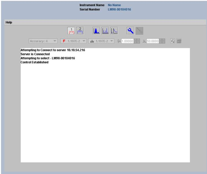
This is the measurement page where most of your time will be spent. From here you can access any of the measurement modes, filament control and diagnostics.
