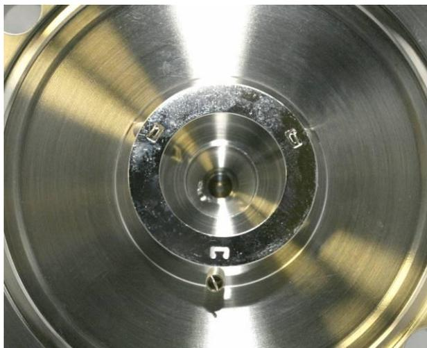
3. From the side without a spring fitted, slide the Ceramic Coupling under the Retaining Ring, paying attention to the couplings orientation, which should be with the shouldered face uppermost.
