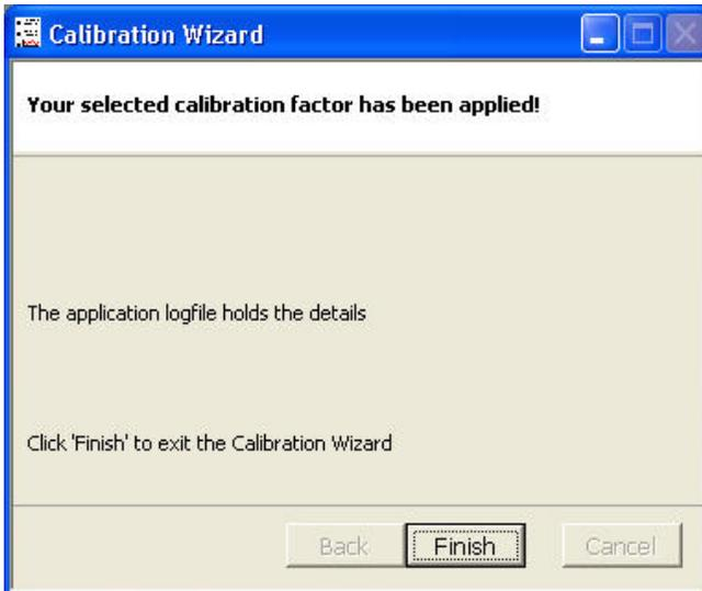
If the new calibration is applied then details will be stored in the application log file Process.xml in the Process Eye\Logs directory
