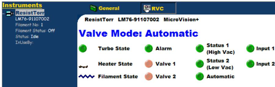
Most of the on-screen indicators are duplicated and mimic those on the front panel with the exception of INPUT1, INPUT2 and VALVE MODE which are displayed here only.
