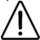
The Exclamation Mark (ISO 3864, No.B.3.1) refers to the need to disconnect the unit from the mains supply before removing the top cover.
