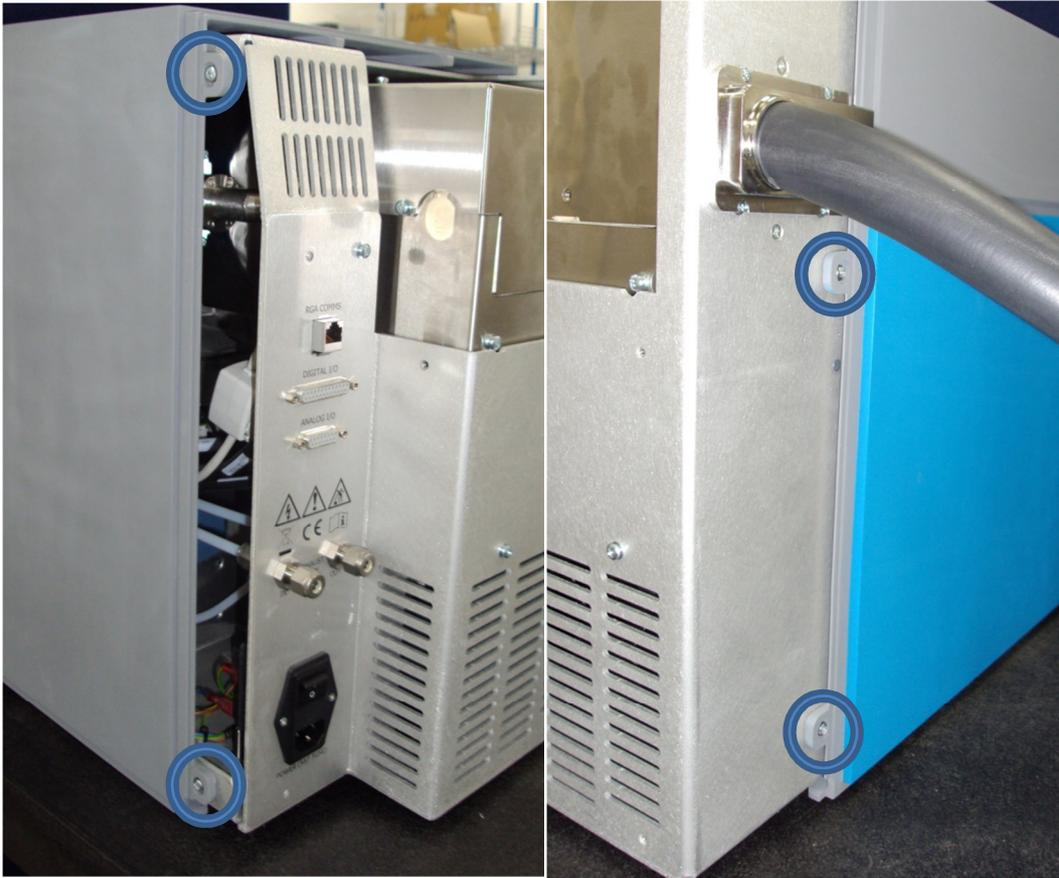
**Illustrations 4a & b. Removal of the front panel is required to access the mass filter for source maintenance.**
