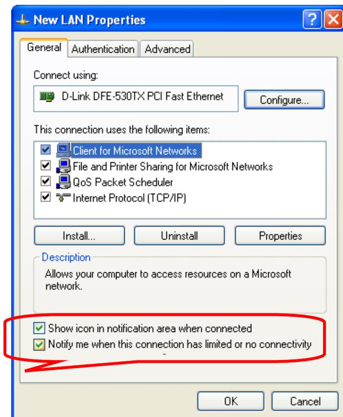
Check the options shown above. Your network connection status is now displayed in the task-bar, near the clock. Mouse-over the icon to check the status of the connection.
