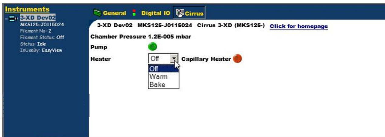
The multiplier detector will be unavailable during baking and for a period afterwards while the system cools down.
