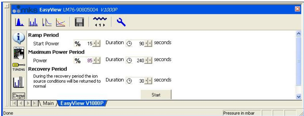
When EasyView degasses an ion source it ramps up to full power over a user defined period of time. It then maintains that power for a further period. When degas is complete it resets the ion source conditions to 'normal' and waits for a period of time during which the temperature of the source can stabilize.
