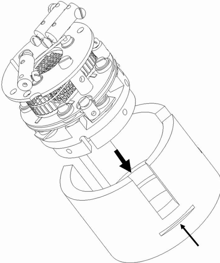
Note the orientation of the source assembly when inserted into the jig. Align the extract plate's barrel connector with the alignment indicator on the jig.
