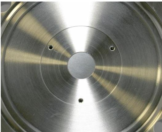
Without disturbing the new Orifice Disk, carefully re-fit the tool guide to the inlet flange. Once the guide is secured, check again that the new Orifice Disk is lying squarely in the tapered hole. If not, it must be re-positioned.
