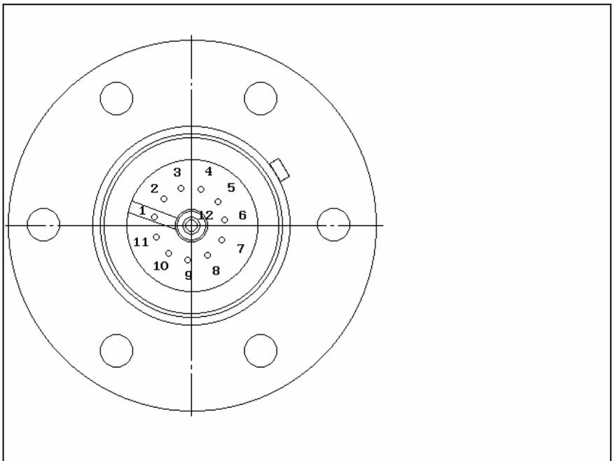
*Figure 8 Analyser pin configuration*
