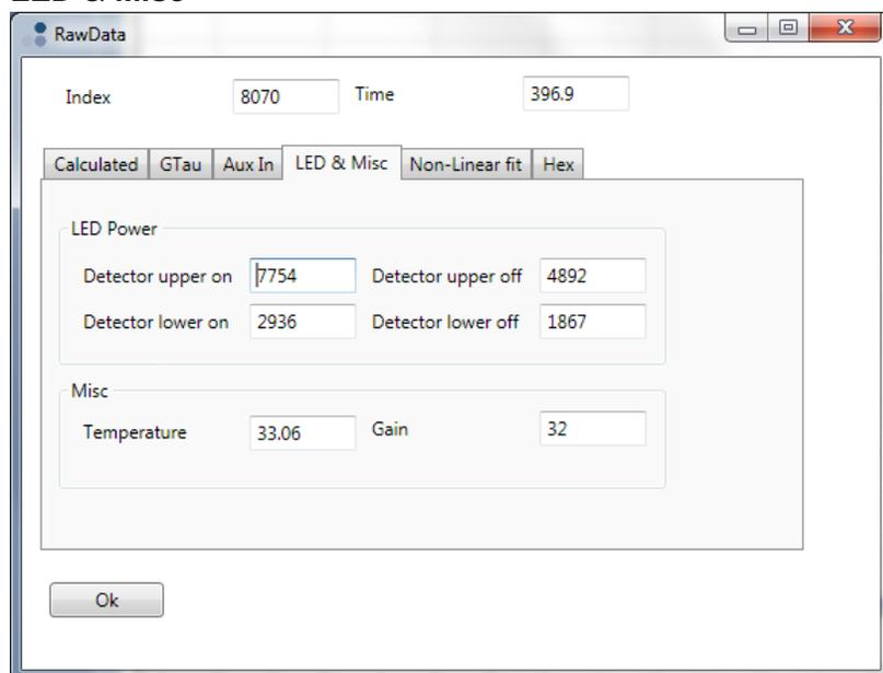
The LED Power values are 16bit A2D readings of the upper and lower photodiodes when the LEDs are high (On) or low (Off). When a wafer has just been removed, for a given configuration these should remain constant.
