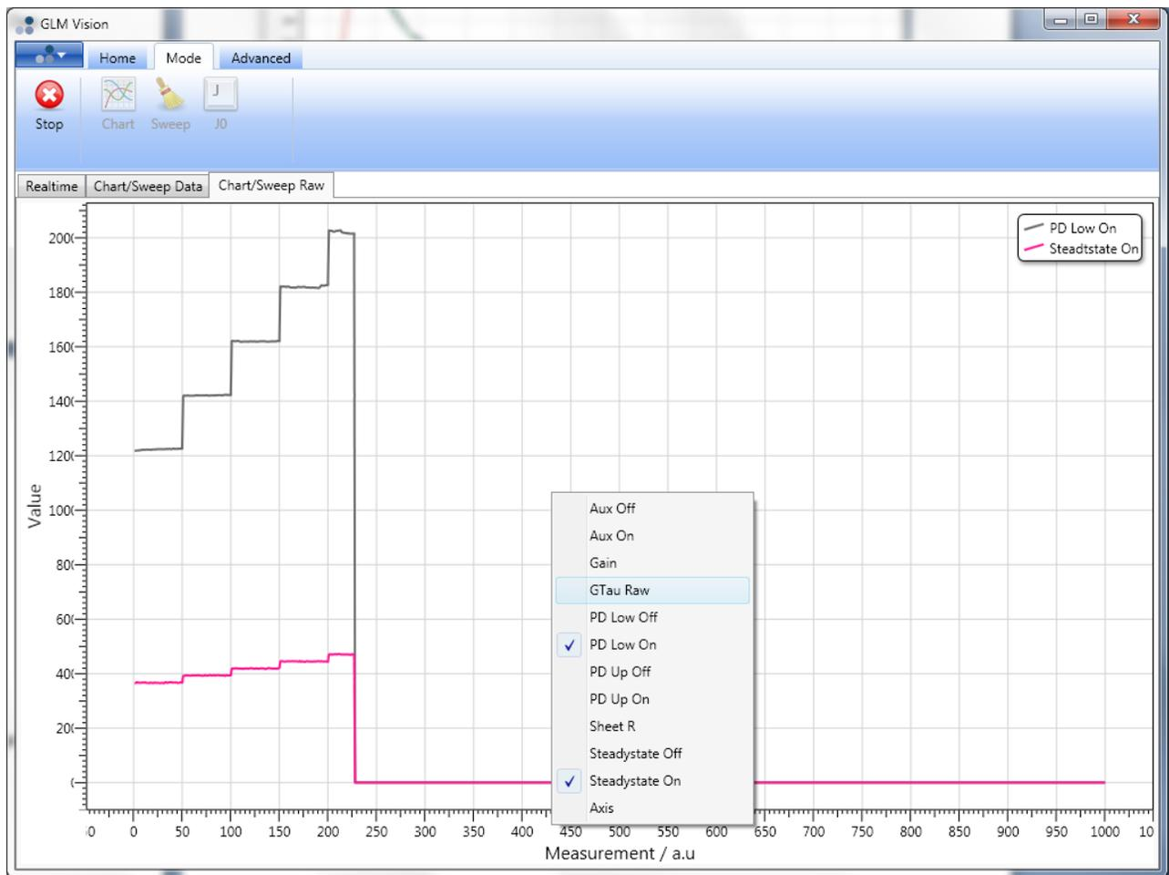
NB: When collecting Sweep data it is advisable to use a fixed Gain as step changes in gain are not then visible in the sweep data.
