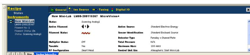
configuration of the hardware you will have tabs across the top for General, Ion Source, Tuning, Digital I/O, RVC and Cirrus. Click on the appropriate tab for the information that you want to view.
