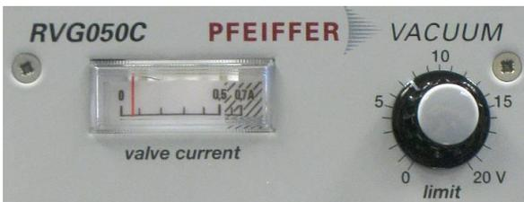
An easy indication of the full closure of the valve is to keep an eye on the Air peak and the voltmeter. Once the air peak has decreased to the base-line and the voltmeter reads zero, we can assume the valve is closed.
