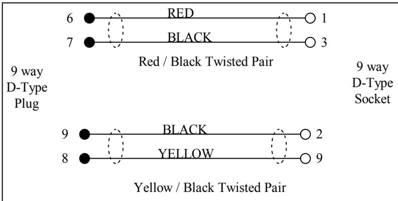
Figure 7 RS422 cable connections
