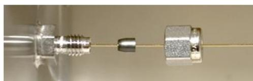
6. Carefully slide the fused silica tube down the capillary assembly away from the inlet flange and remove the nut and ferrule.
