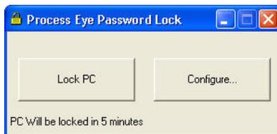
To lock the PC, click **Lock PC**. If you do nothing (i.e. no mouse actions or key presses) the PC will be locked after 5 minutes.
