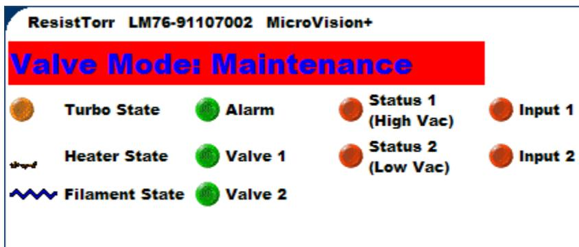
Maintenance Mode can be activated only by turning the key switch on the front of the RV2C to the **INTERLOCKS OFF** position.
