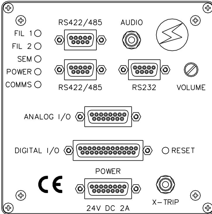
Figure 2 Microvision Plus connector layout
