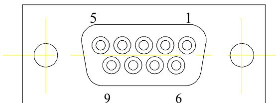
*Figure 4 RS232 connector (9 way D-Type socket)*
