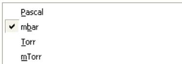
A "tick" in the selection indicates the currently used pressure unit. All pressure axes will also be labeled with the current unit.
