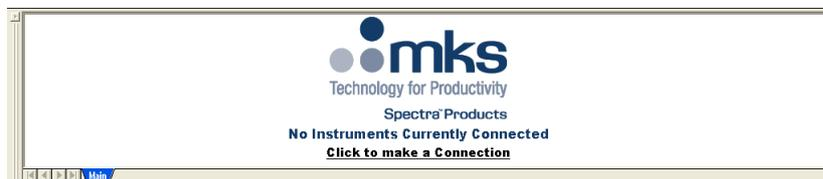
If there are no instruments connected, or if the system is not set up for exclusive access to any instruments, then the page will appear as above.
