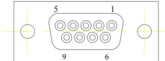
Figure 6 RS422 connector (9 way D-Type socket)
