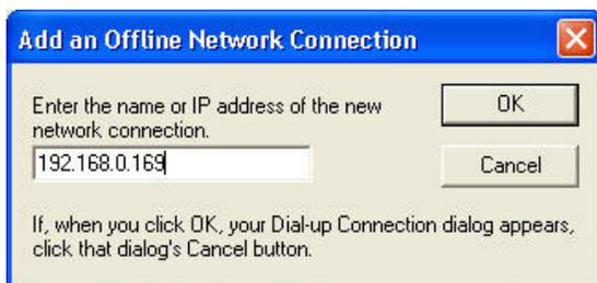
In this dialog, enter the IP address of the remote PC, or providing your network has "DNS Lookup", you can simply type the network name of the remote PC.
