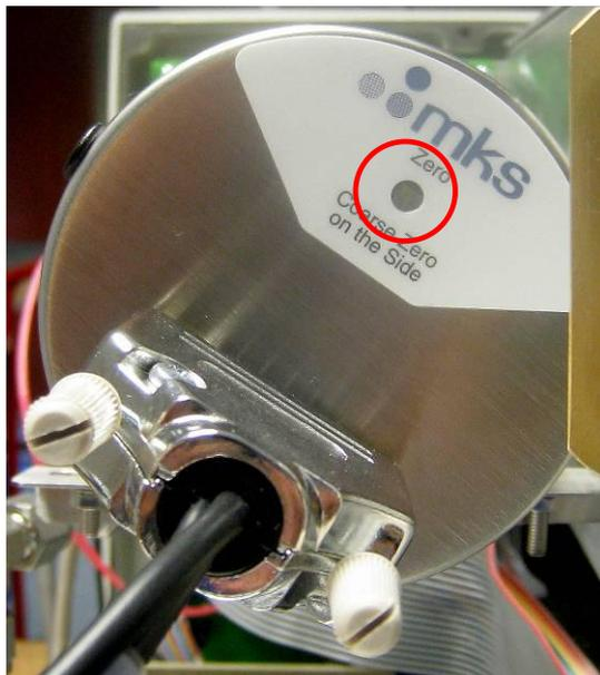
If a zero cannot be achieved with the fine adjustment, there is a coarse adjustment on the side of the gauge.
