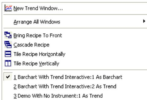
The bottom section of the pull down list contains a list of the currently open views. The current active view is indicated by a tick next to it.
