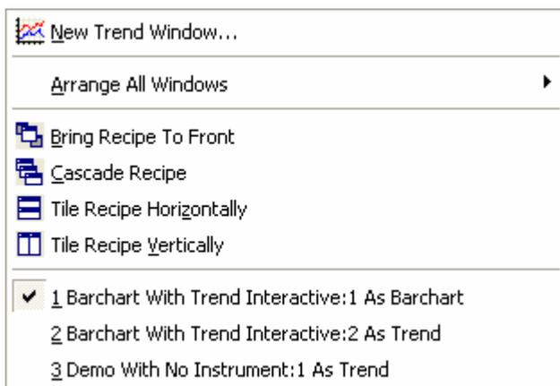
The bottom section of the pull down list contains a list of the currently open views. The current active view is indicated by a tick next to it. To make a different view active, click on that view. As well as making this the active view it will also bring the view to the front.
