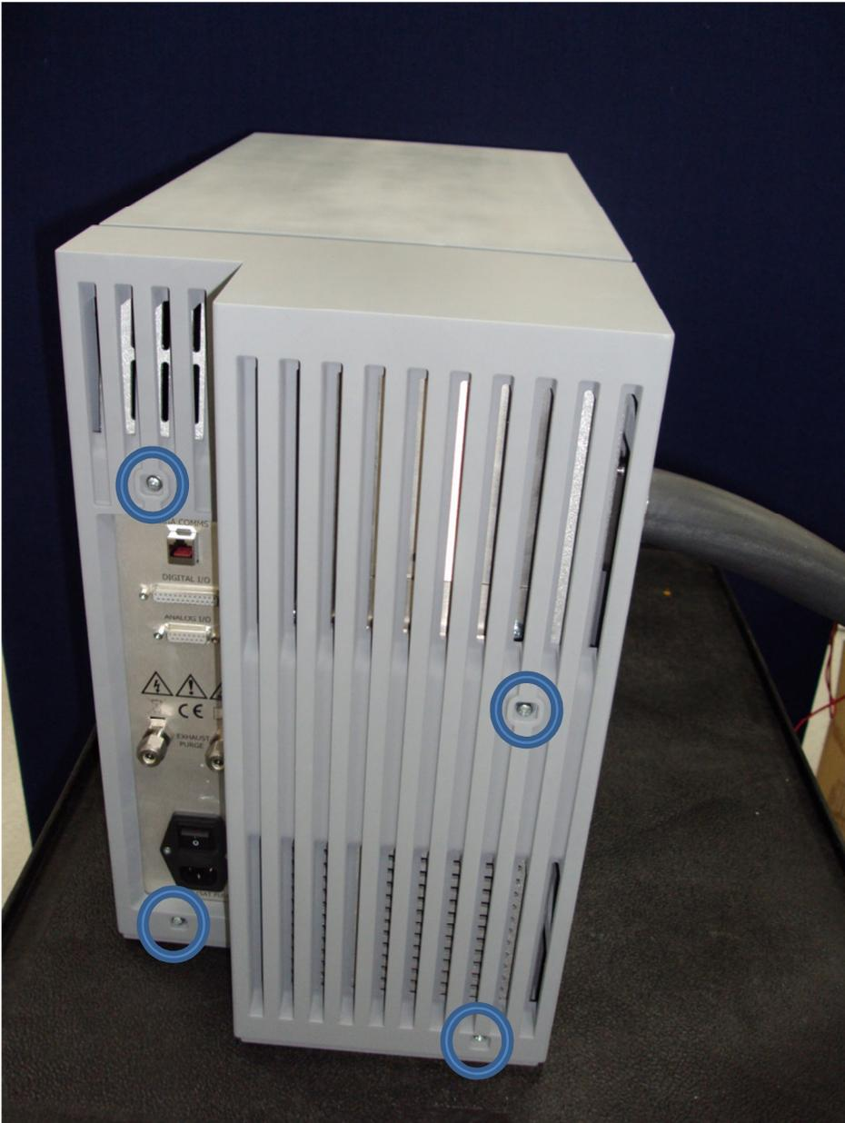
**Illustration 3. To access the rear of the instrument, required for changing the capillary and orifice disk, the rear panel must be removed. This is done by removing the four screws and pulling the panel backwards until clear of the instrument.**
