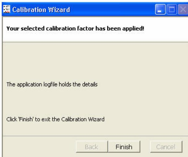
If the new calibration is applied then details will be stored in the application log file Process.xml in the Process Eye\Logs directory
