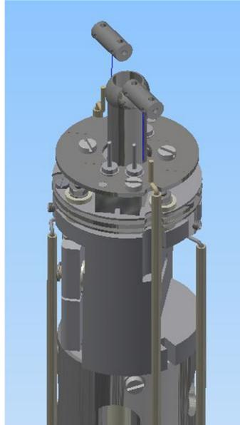
Illustration 20. Remove barrel connectors
