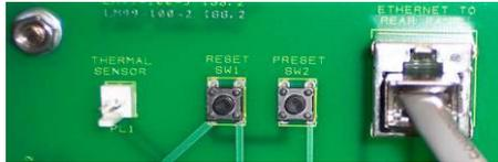
With power applied to the Cirrus, press the “reset” button and immediately press and hold the “preset” button until a “beep” is heard from the unit.
