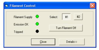
The "Filament Control" dialog now changes to show the **Filament Supply** and **Emission OK** are both good and that the filament has not been **Tripped**.
