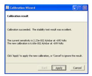
Details of the previous and current calibration will be displayed, click **<Apply>** to apply the current calibration.
