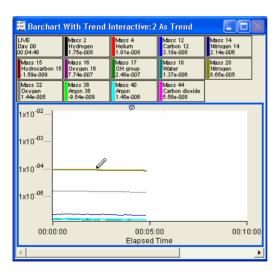
Each annotation added will be marked by a symbol along the top of the trend. If you move the cursor over this symbol, the text will be displayed as a tool tip.
