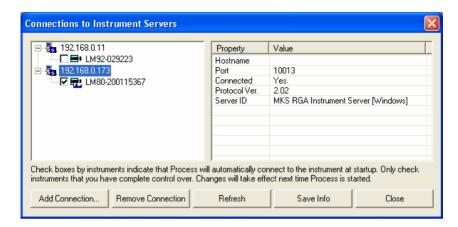
To remove a connection, simply highlight the connection that is no longer required and click on the **<Remove Connection>** button.
