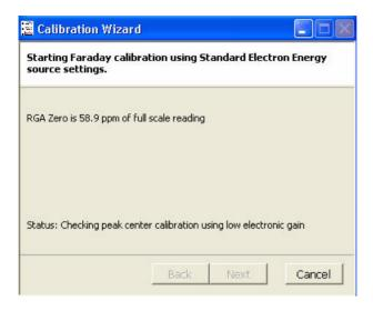
The first step is to measure the zero and check the mass alignment
