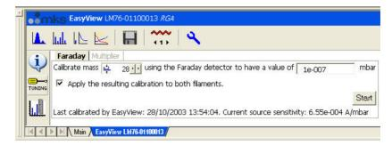
The date of the calibration and sensitivity value will then be displayed at the bottom of the EasyView window.
