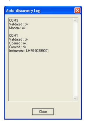
The auto discovery report lists all the com ports checked on the system. For each Com port the results of the tests are displayed along with the serial number of any instrument found on that port.
