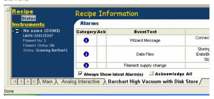
In the status window, the tabs for the running recipes are displayed. The uppermost tab is the selected recipe. In the above example, **Bar chart High Vacuum with Disk Store** is the selected recipe.
