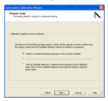
This dialog is used to choose the method employed to perform the calibration. Scaling to an external pressure gauge reading uses the same method as the Faraday calibration, so this example will use the second method which calibrates the multiplier to match the Faraday measurements. Select the appropriate option and click **Next>**.
