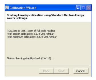
When the peak maximum and peak center readings have been taken the stability is checked.
