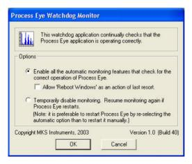
The watchdog can be temporarily disabled by selecting the second option box and can cause windows to reboot if the **Allow Reboot Windows** checkbox is checked. However the program will automatically restart when Windows reboots, or if Process Eye is restarted.
