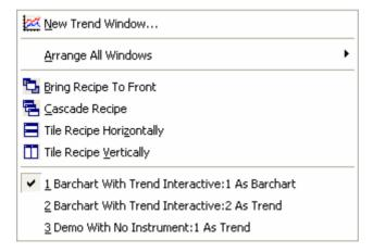
The bottom section of the pull down list contains a list of the currently open views. The current active view is indicated by a tick next to it. To make a different view active, click on that view. As will as making this the active view it will also bring the view to the front.
