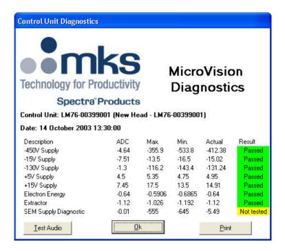
The diagnostics report shows the details of all measurements made on the power supplies within the instrument, giving the upper and lower limits for each individual supply voltage and displaying a "Pass" or "Fail" result.
