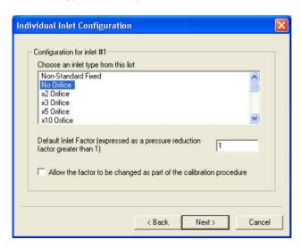
Depending on the inlet chosen, the factor for the first inlet can be set. The inlet factor is always greater than, or equal to 1. If the inlet halves the pressure then the inlet factor is 2 for example. We do not currently support inlets that cause an
