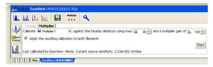
Select the multiplier setting to be calibrated from the drop down list, the mass to calibrate on and the multiplier gain required. The multiplier will be calibrated at the mass chosen, so that the pressure reported in faraday and multiplier at this mass will be the same.
