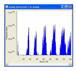
The alternative is the **Trend** view, where a variable versus time can be plotted.
