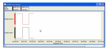
This option is only useful for displaying digital data. In the above example, there are two digital input channels with both channels configured to **Draw stepped**".
