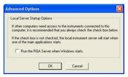
If network access for the local instrument is required, check the **Run the RGA Server when Windows starts** option. This will start the server program whenever Windows starts. If the option is not checked then the server program will only start when one of the MKS RGA Applications such as Process Eye Professional starts
