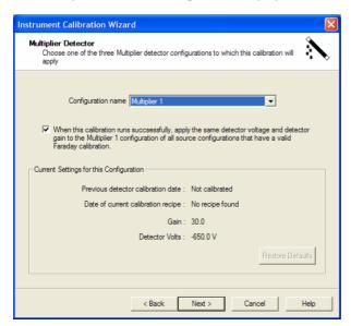
This dialog is used to choose which multiplier detector configuration the calibration will apply to, and also displays the details of any previous calibrations. Click **<Next>** to continue.
