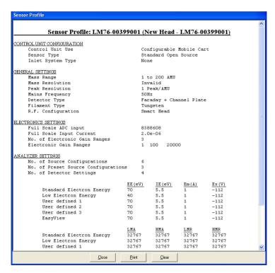
The "Sensor Configuration" report shows all the configurable settings for the instrument. These settings can be checked against the report included with the instrument when shipped, in case adjustment is required.
