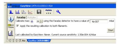
Pick a mass to calibrate on and enter the partial pressure of that mass. To start the calibration click on **<Start>**
