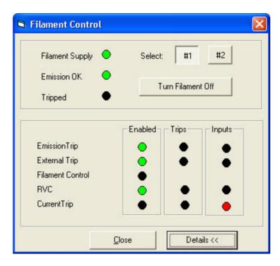
In the above example the filament switched on OK so the **Filament Supply** and **Emission OK** indicators are green.
