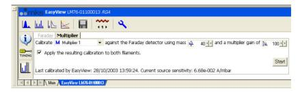
The date and sensitivity of the current calibration will be displayed at the bottom of the EasyView window
