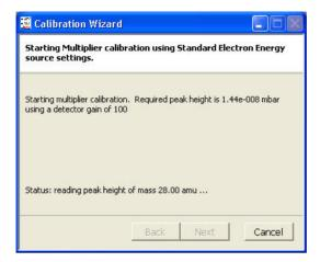
Once the multiplier voltage has been adjusted, the recipe will perform another twelve scans to check the stability of the calibration.
