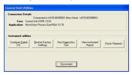
This page gives details of the downloaded software versions and allows various functions to be performed on the instrument. **Configure Digital IO** and **Run Diagnostics** can also be performed directly from the **Advanced>** pull down menu
