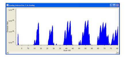
In this view, the first and last masses measured are shown on the X-axis along with the scan number.
