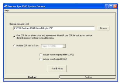
This will bring up the System Backup dialog, choose the location and name for the backup file. To make a backup spanned across a number of disks, click the **Multiple Zip files to fit** option and select the type of media that the files must fit on. There is a custom size option, simply select and then enter the size of files to be created
