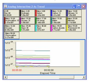
This type of view is more flexible as the data plotted is not necessarily partial pressures, any user variable can be plotted on trend.
