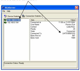
If Process Eye was configured not to pre-connect to an instrument, there would only be an Information connection as shown in the diagram.
