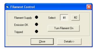
To switch on a filament, select either filament 1 or 2 and click the **<Turn Filament On>** button.
