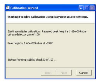
The calibration will perform a zero, measure the peak height in faraday, adjust the multiplier voltage so the peak height in multiplier with the gain specified matches and then check the stability.
