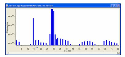
In this case you can see that the Y-axis of the chart is labelled in mBar. To change this to Torr, click on **<Torr>** in the selection.
