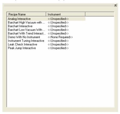
Generic recipes will have an "unspecified" instrument, recipes that do not use an instrument will have "None required" as the instrument.
