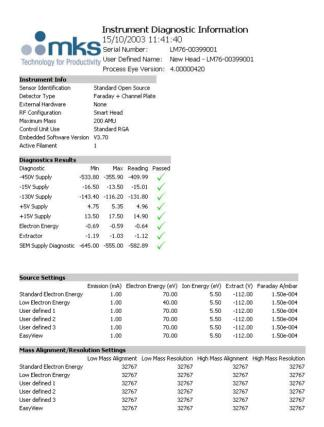
The report contains information about the control unit configuration, source settings and mass alignment/resolution settings as well as power supply levels.
