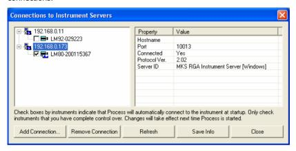
Clicking on the server will provide details about that connection. Clicking on the instrument will provide details about that instrument.
