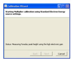
Then the multiplier peak height is measured. The multiplier voltage will be increased or decreased until the multiplier peak height matches that of the Faraday reading.
