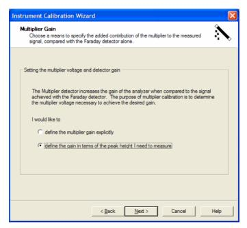
This dialog allows you to choose how you want to define the gain of the multiplier detector. There are two choices; **Define the multiplier gain explicitly,** where a user defined gain setting is used for calibration,
