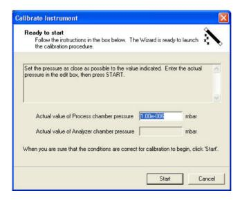
Enter a corrected gas pressure and press **<Start>** to begin the calibration.
