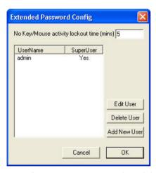
In configure you can create, edit and delete users. You can also change the time without use before the computer is locked. To do this simply enter a number in the to text box.
