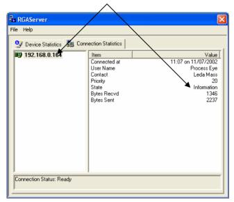
When a recipe is started, a Control connection is made and RGA Server will again display both connections.
