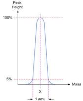
All instruments have the mass alignment and resolution set before leaving the factory. A copy of the tuning numbers will always be included with the documentation. Only small changes to the alignment and resolution should ever be necessary to account for small changes in temperature between the factory and place of operation. If major changes are made to the settings so that peaks are no longer visible, please re-enter the factory defaults to try and recover the peaks.
