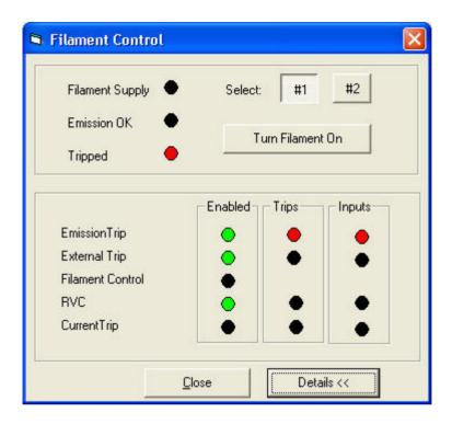
In this example the filament has been tripped off, the **Filament Supply** and **Emission OK** indicators are not lit but the **Tripped** indicator is.
