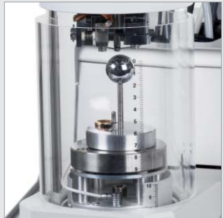
Carbon Rod Evaporation by indirect evaporation using a shadowing sphere.
