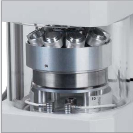
High vacuum sputtering using the planetary drive stage, SEM specimen mounts, stubs and quartz head.
