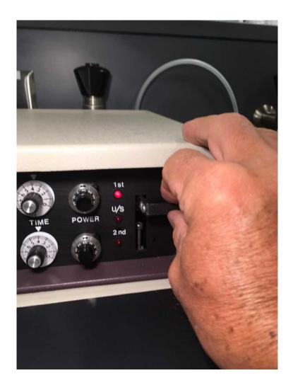
**4.3** Next reposition (using the chessman mouse) to the 2<sup>nd</sup> and final termination bond position. Once you are in contact hold this position until the front panel "LED" indicator has switched back to the 1<sup>st</sup> bond position mode.
