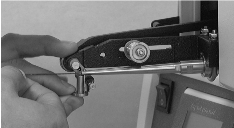
Figure 5-1: Wedge Installation Using the Setup Gauge -4523D, 4523AD with 30°/45° Wire Feed, 0.75" Drop
