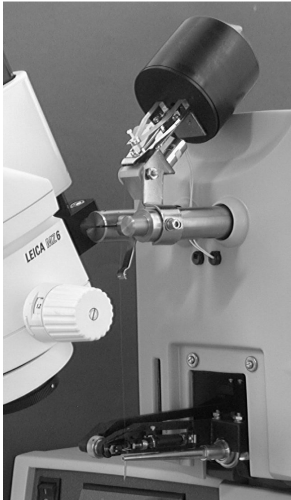
Figure 5-10: Wire Loading of 2" Spool - Vertical Wire Feed
