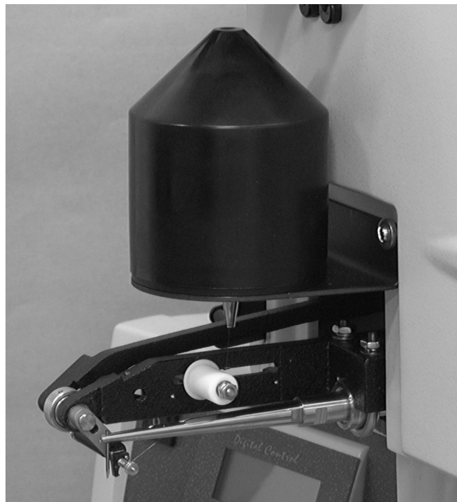
Figure 5-8: Wire Loading of 2" Spool - 30°/45° Wire Feed
