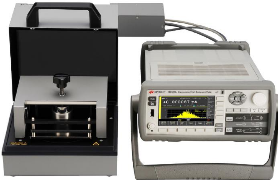
Figure 11. B2987A and N1424 configured to make resistivity measurements
