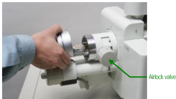
Withdraw the exchange rod
