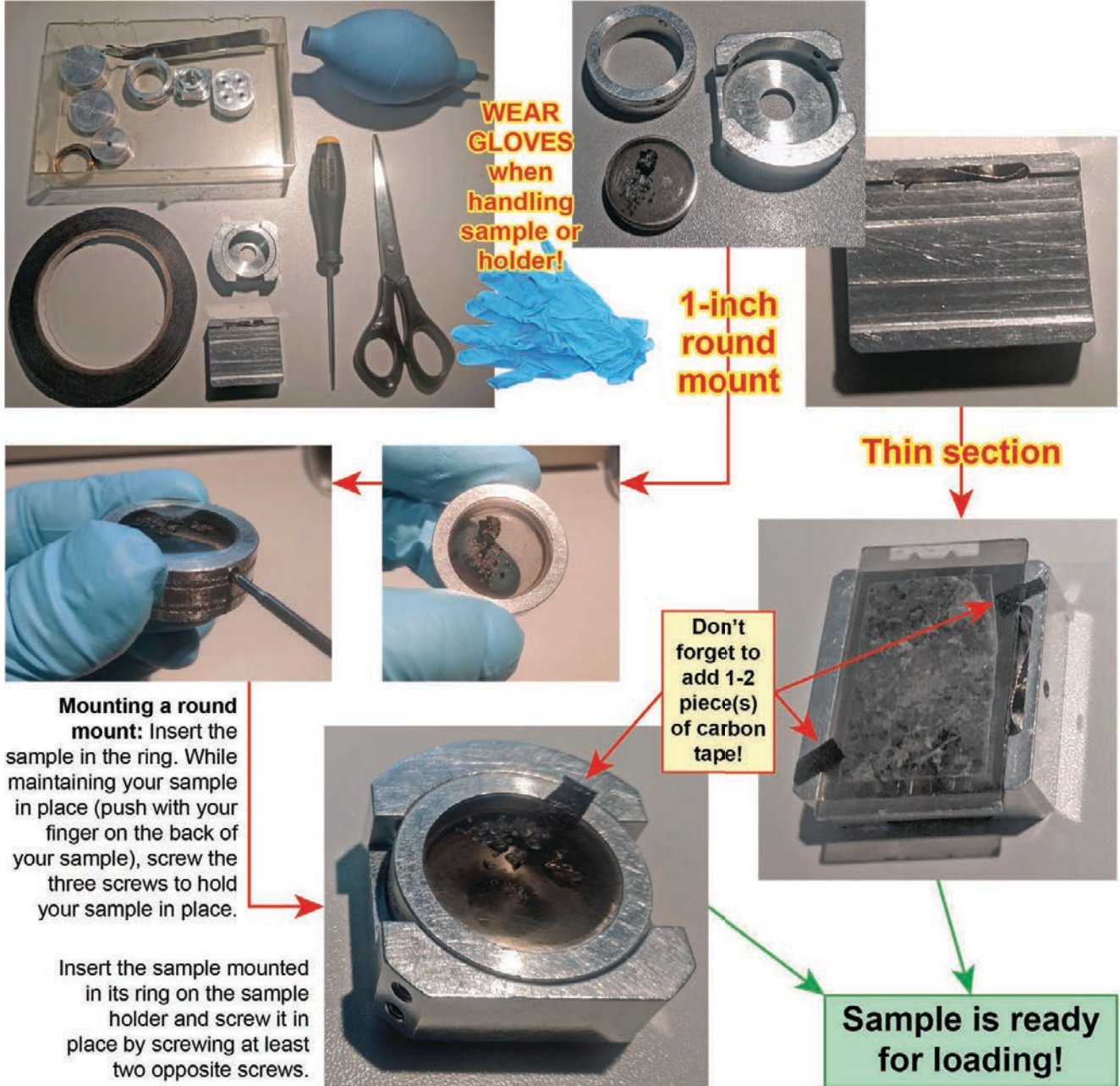
Figure 9. Preparing the sample holder (for thin section or for 1" round mount).
