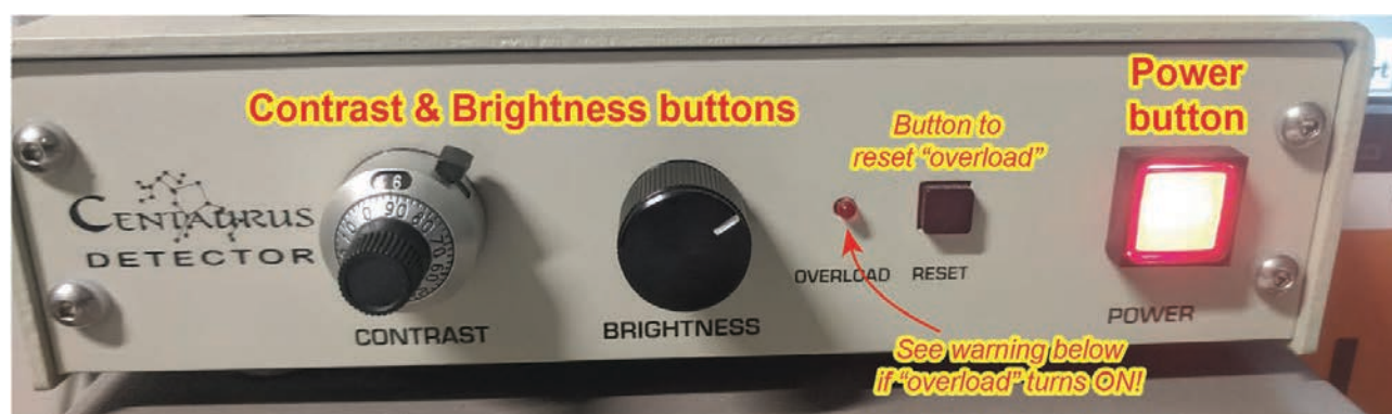
Figure 17b. Control box for the “Centaurus” CL detector.
