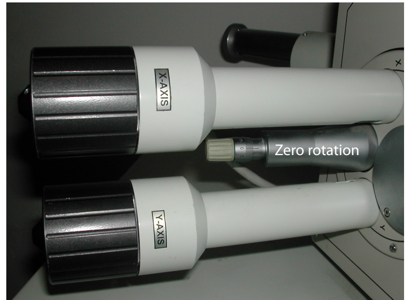
Note - Rotation must be kept at zero to maintain orientation reference frame constant for mapping
