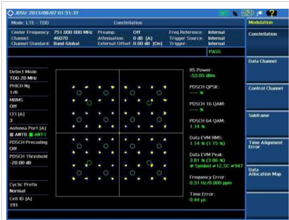
LTE - TDD Constellation Measurement Screen
