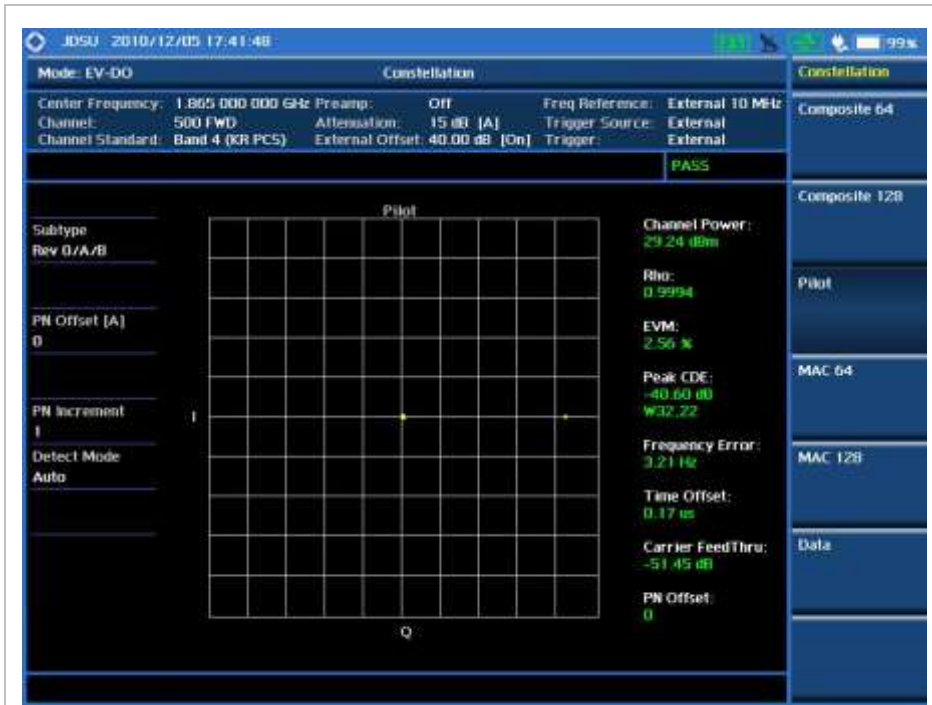
EV-DO Constellation Measurement Screen (Pilot)
