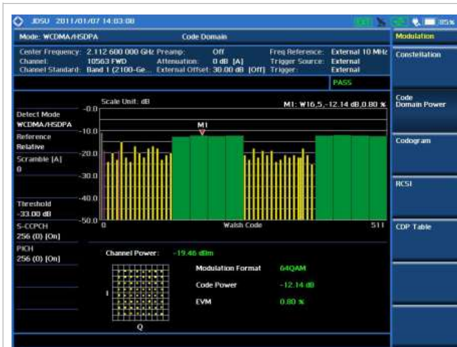
WCDMA Code Domain Analysis Full Screen (with Constellation)
