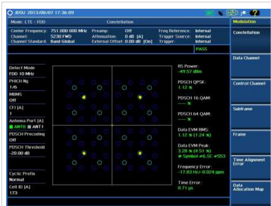
LTE - FDD Constellation Measurement Screen
