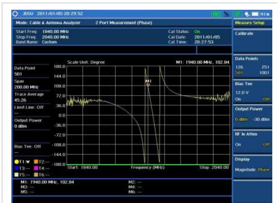
2 Port Measurement (Phase) Screen
