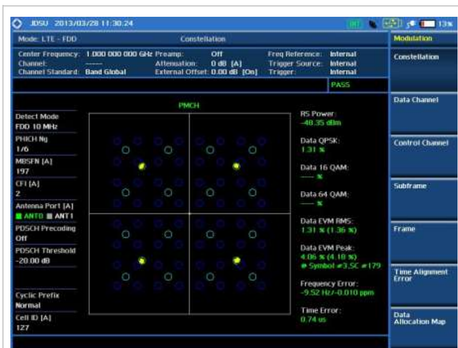
LTE - FDD Constellation Measurement Screen (MBMS On)
