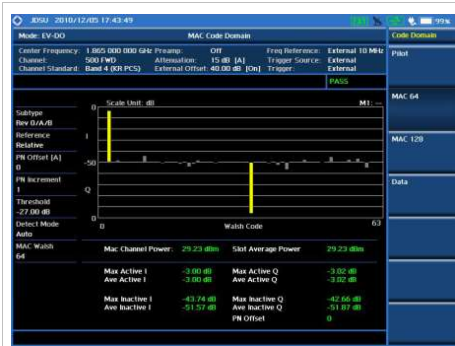
EV-DO Code Domain Power Analysis Measurement Screen (MAC 64)
