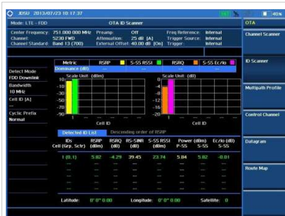
LTE - FDD OTA ID Scanner Measurement Screen
