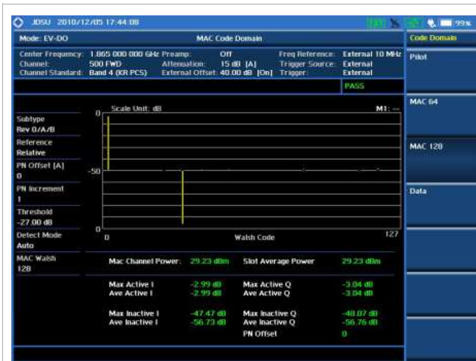
EV-DO Code Domain Power Analysis Measurement Screen (MAC 128)
