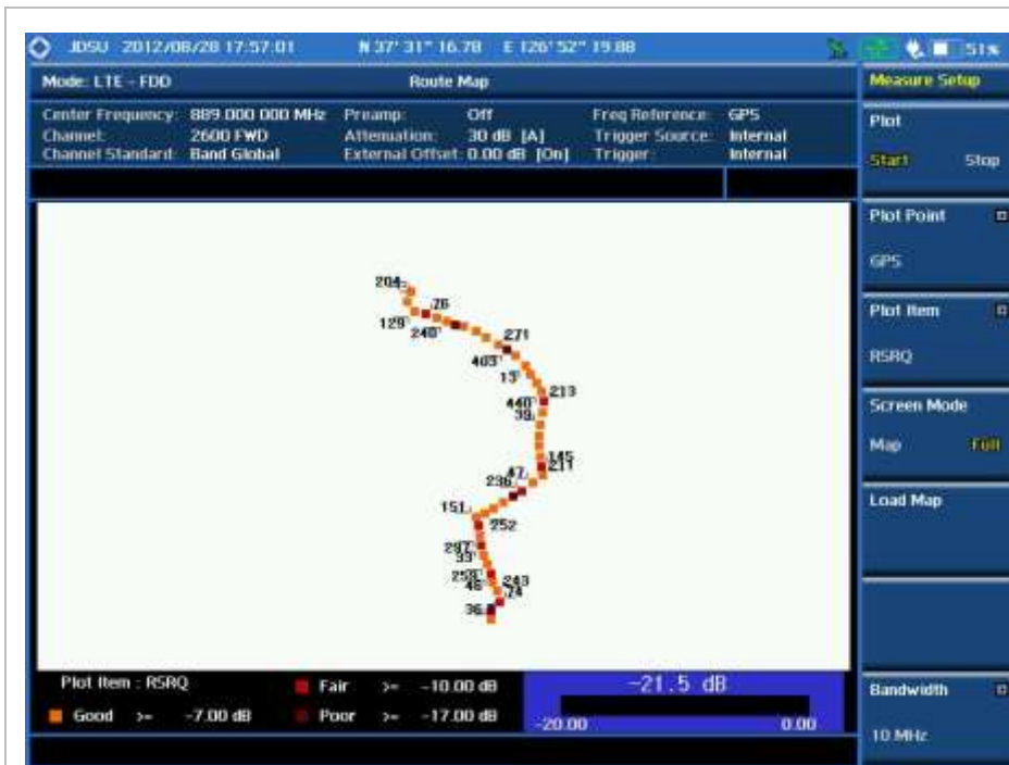
Route Map Measurement Screen (Full View)
