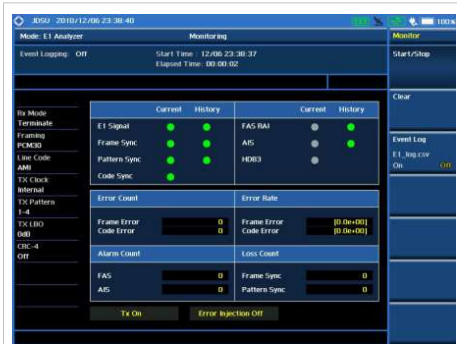
E1 Transmission Monitoring Screen
