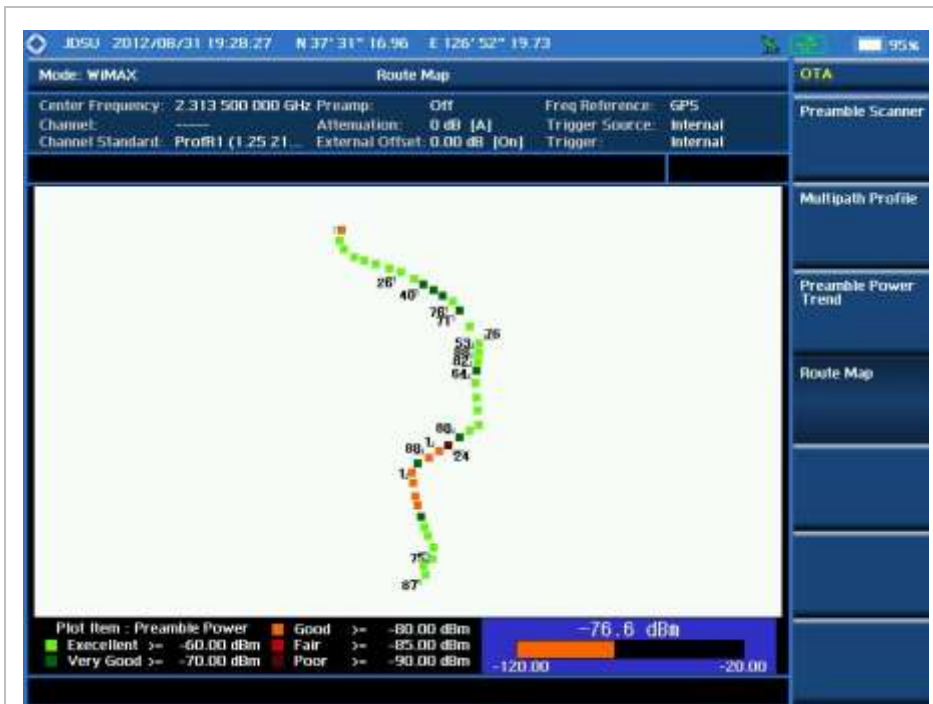
Route Map Measurement Screen (Full View)
