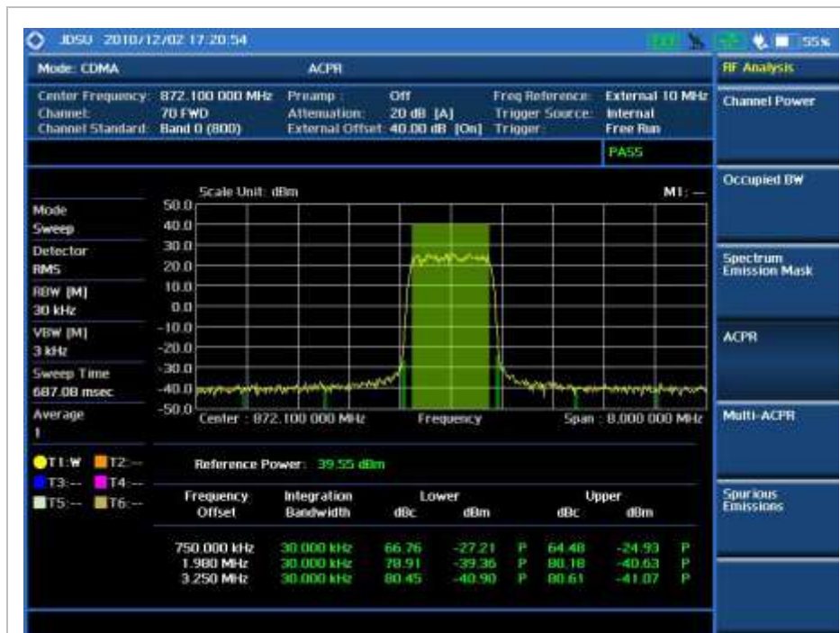
CDMA ACPR Measurement Screen
