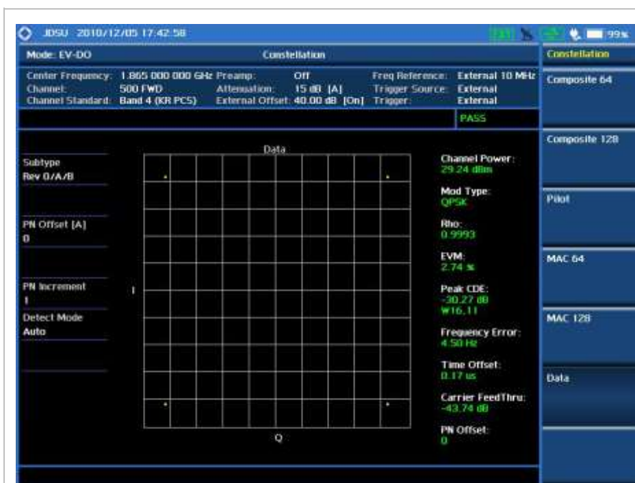
EV-DO Constellation Measurement Screen (Data)
