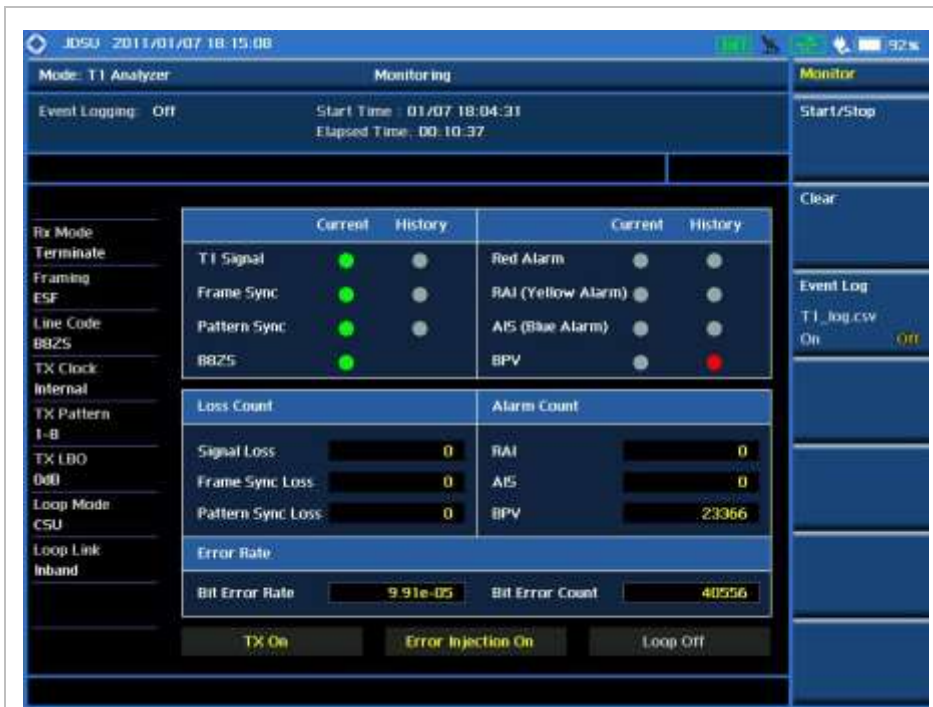
T1 Transmission Monitoring Screen
