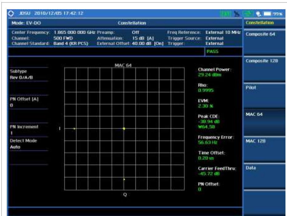
EV-DO Constellation Measurement Screen (MAC 64)
