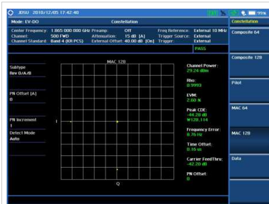
EV-DO Constellation Measurement Screen (MAC 128)
