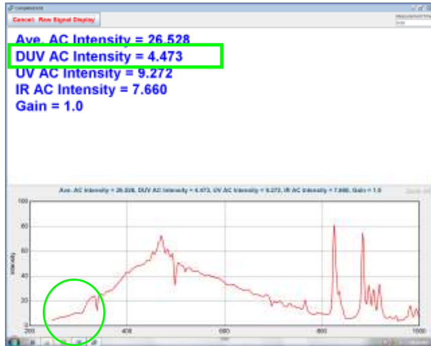
Figure 4-4. Filter 4 with iris closed to avoid Overloading the Spectrometer.
