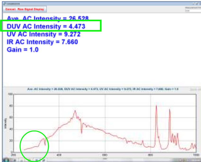
Figure 10-11. Filter 4 with iris closed to avoid Overloading the Spectrometer.
