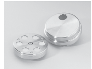
Crystal retainer assembly and standard stainless steel cover
