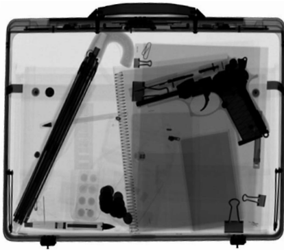
[Figure 2-1] Imaging example of baggage inspection equipment
