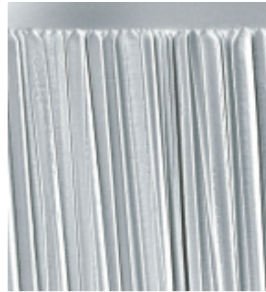
Figure 11: The needle-like crystal structure of CsI
