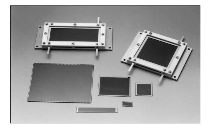
A microchannel plate (MCP) is a secondary electron multiplier consisting of an array of glass capillaries (channels) fused into the form of a thin plate. Each channel has an internal diameter of 6  $\mu$ m to 25  $\mu$ m and works as an independent electron multiplier, making possible the detection and amplification of two-dimensional information.
