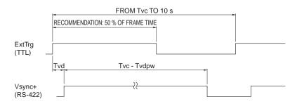
Hsync+, Pclk and Data 1-12 are the same as internal trigger mode.
