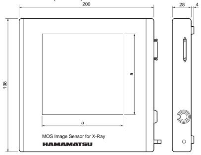
Top cover is made of aluminum 1.0 mm thick.
