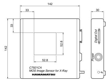
Top cover is made of aluminum 1.0 mm thickness. Weight: 1.37 kg
