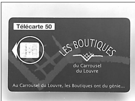
▲ Telephone card with built-in IC chip (inside circled area)
