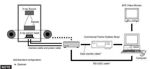
• The C7390 X-ray line sensor camera consists of a sensor head, sensor control unit and cables. Image display equipment should be ordered separately.
