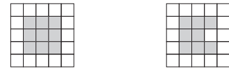
This is defined as defect cluster. This is not defined as defect cluster.
