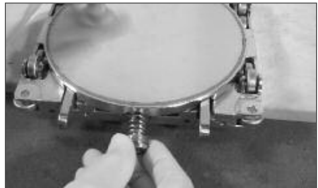
Install the gate spring
