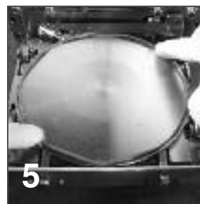
5 Press straight down without twisting the O-ring.
