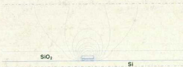
Fig. 9. Parasitic capacitance calculation by FCAP2 for polysilicon line used in HQMOS circuits. Field oxide thickness = 0.4 \mu\text{m} , polysilicon thickness = 0.4 \mu\text{m} , and line-width = 1.8 \mu\text{m} .
